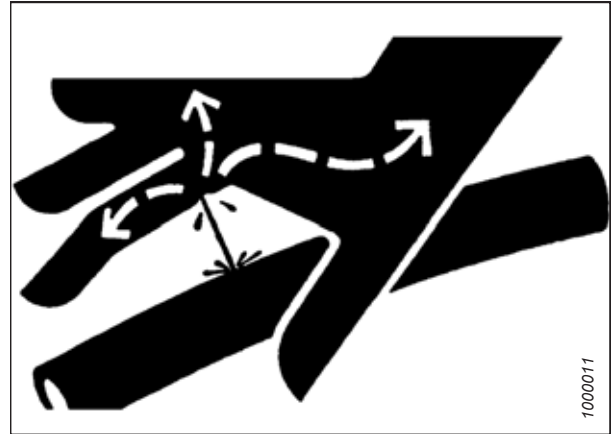
Figure 5.28: Hydraulic Pressure Hazard
