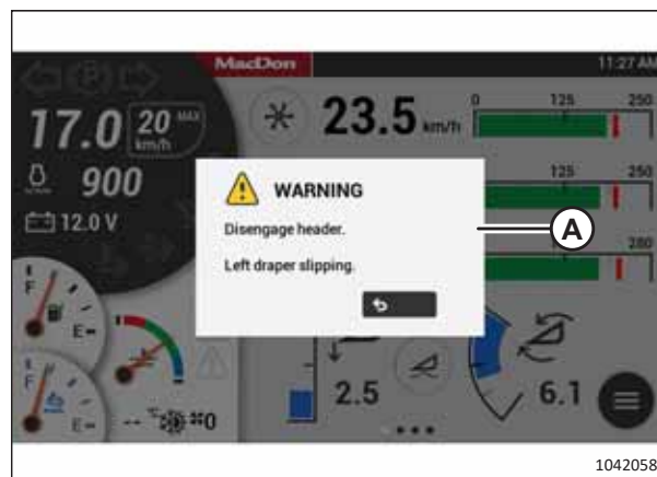
Figure 4.431: Draper Slip Warning
