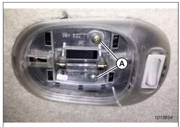
Figure 5.226: Cabin Dome Light with Cover Removed
