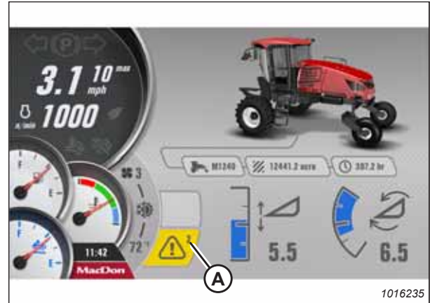
Figure 3.130: Telltale Icon – Multiple Faults Detected
