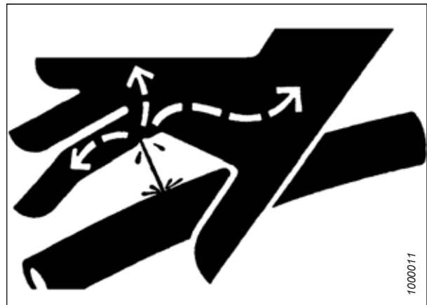
Figure 5.66: Hydraulic Pressure Hazard
