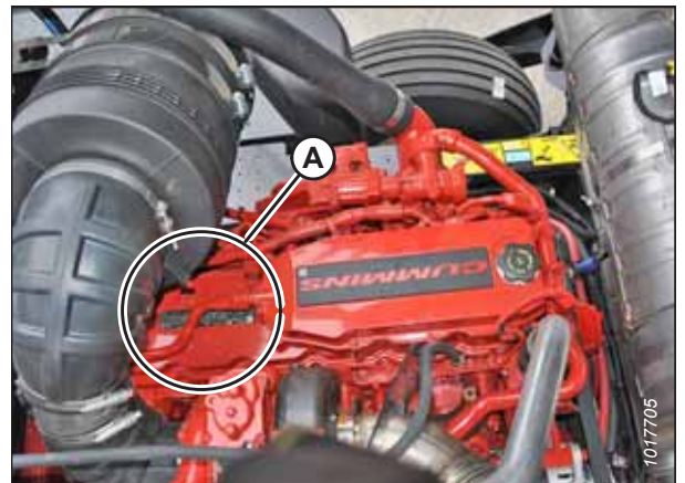
Figure 2: Engine Serial Number Location
