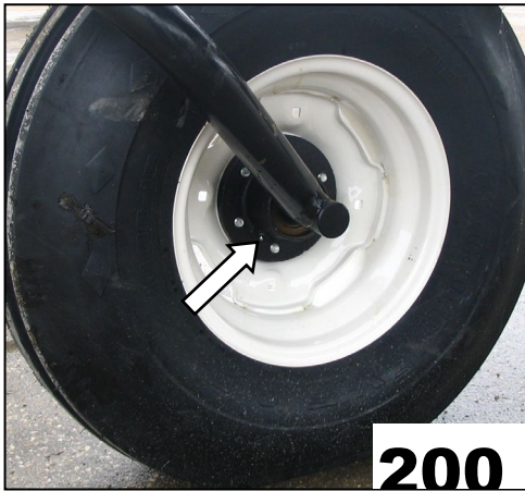
FORMED CASTER WHEEL BEARING 1 PLACE (BOTH WHEELS)
