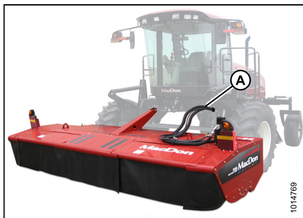
Figure 4.215: Header Drive Hydraulics
