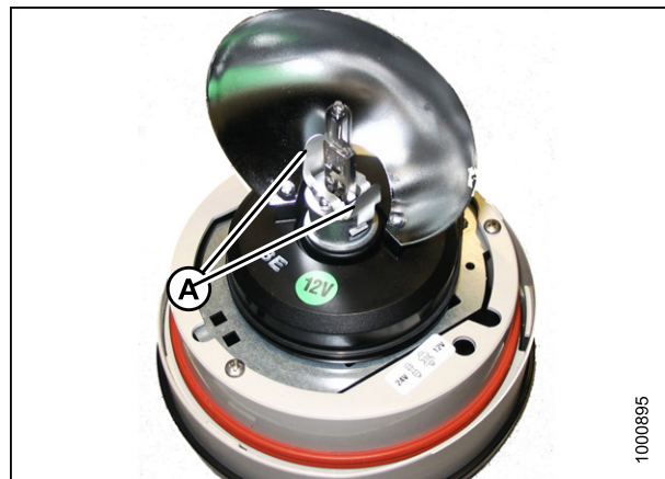
Figure 5.159: Beacon Lamp Assembly
