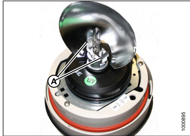
Figure 5.162: Beacon Lamp Assembly
