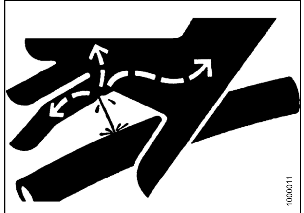
Figure 5.177: Hydraulic Pressure Hazard
