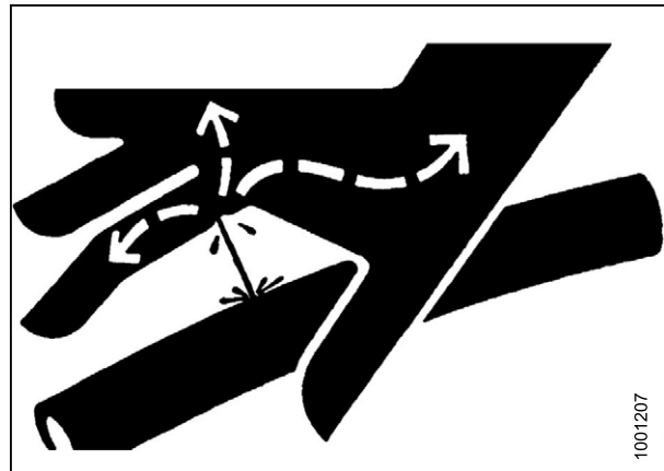
Figure 1.12: Hydraulic Pressure Hazard
