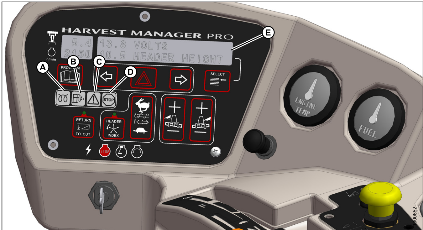
Figure 3.69: CDM Engine Warning Lights
