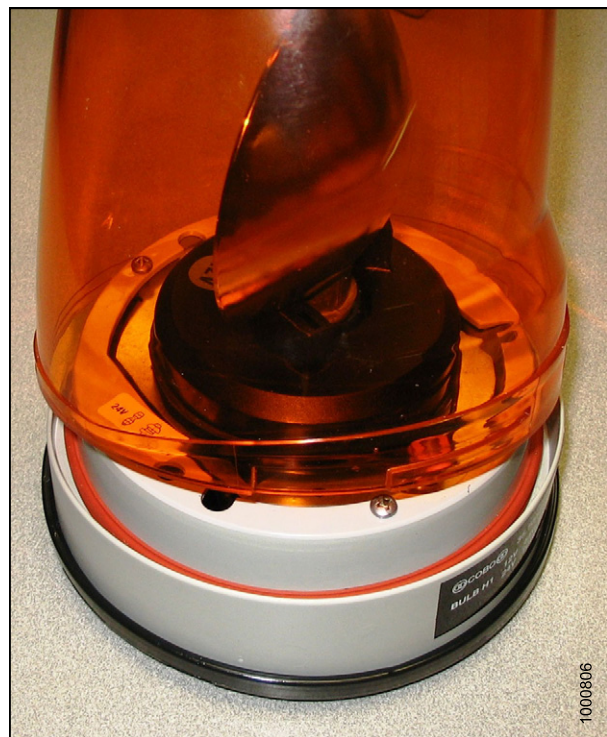
Figure 5.163: Beacon Lamp Assembly
