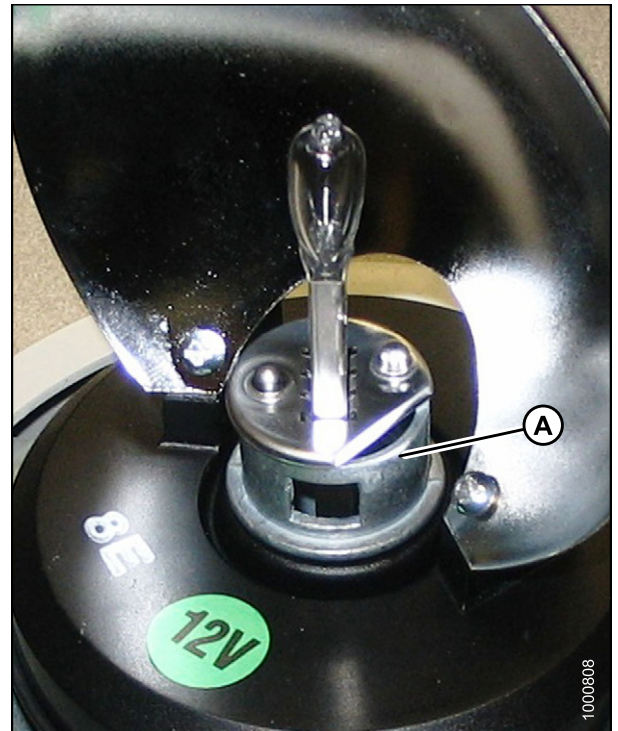
Figure 5.161: Beacon Lamp Assembly
