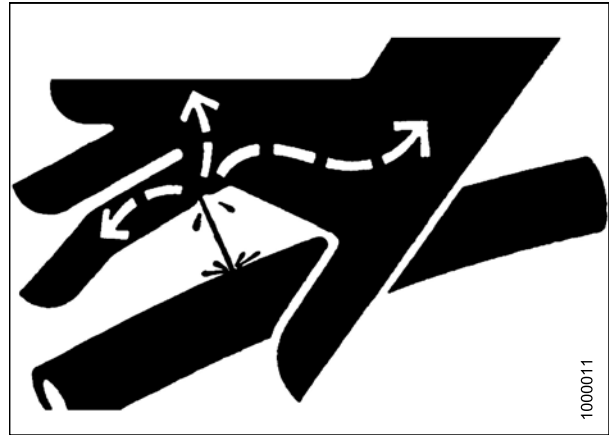
Figure 5.179: Hydraulic Pressure Hazard
