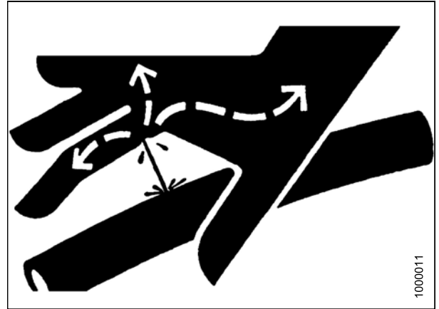
Figure 5.192: Hydraulic Pressure Hazard
