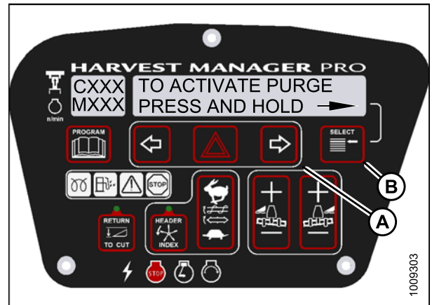
Figure 3.215: M155 Hydraulic Purge
