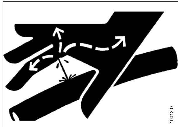
Figure 1.12: Hydraulic Pressure Hazard
