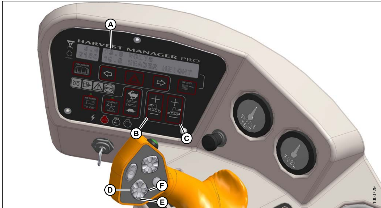
A - CDM Display B - Left Float Adjustment C - Right Float Adjustment D - Header Tilt Down E - Header Lower F - Header Tilt Up
