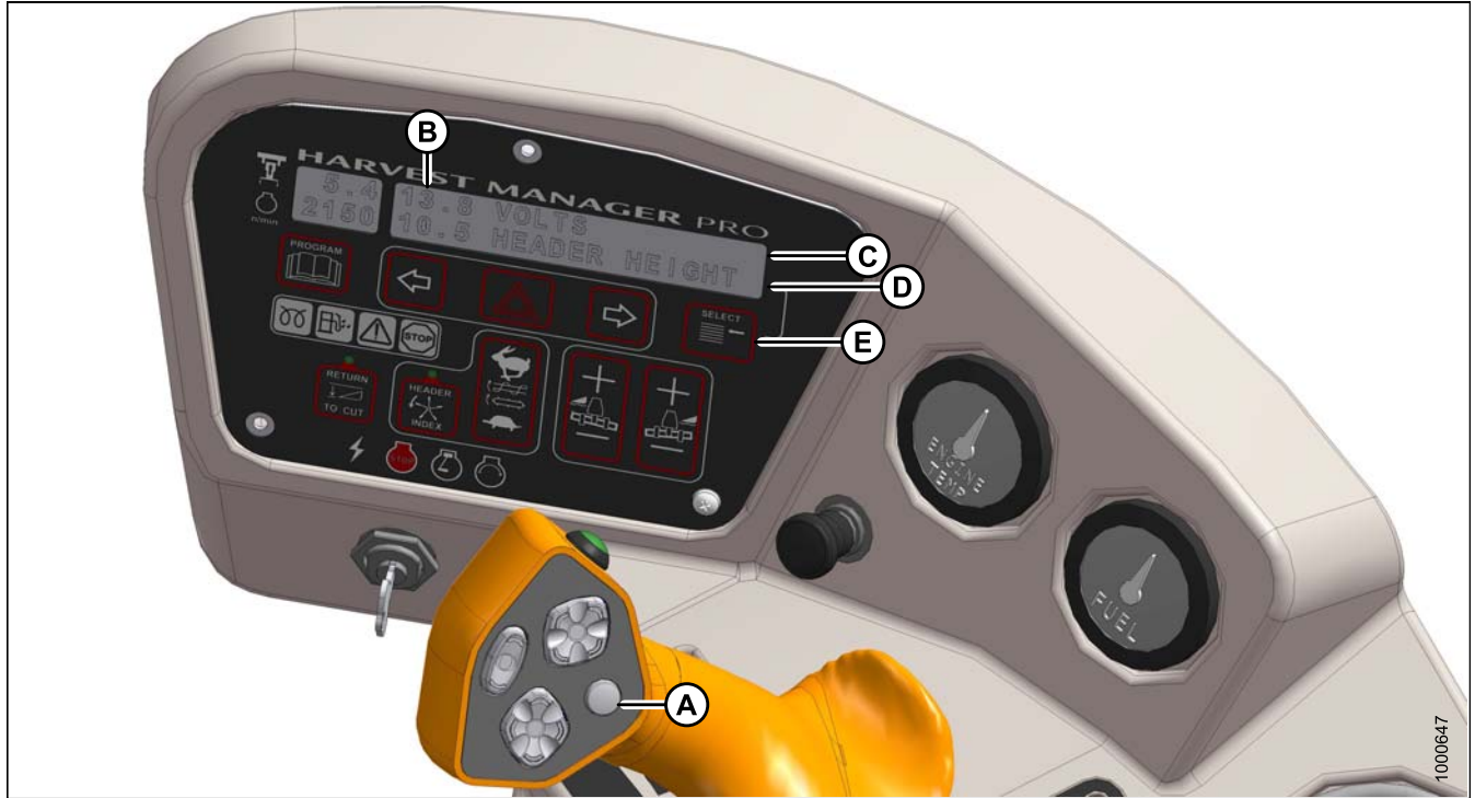
Figure 3.60: CDM Operating Screen
