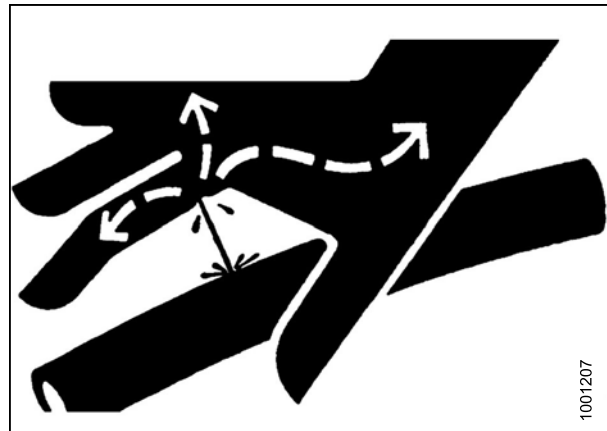
Figure 1.12: Hydraulic Pressure Hazard
