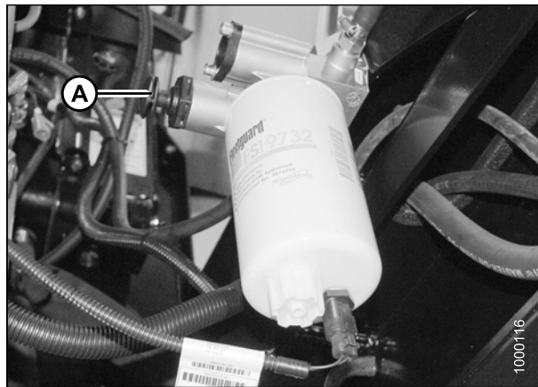
Figure 5.78: Primary Fuel Filter
