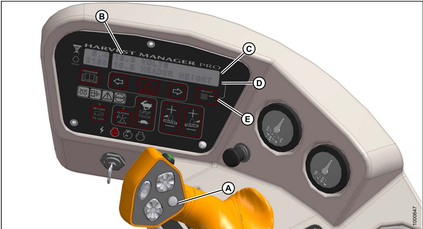
Figure 3.67: CDM Operating Screen
