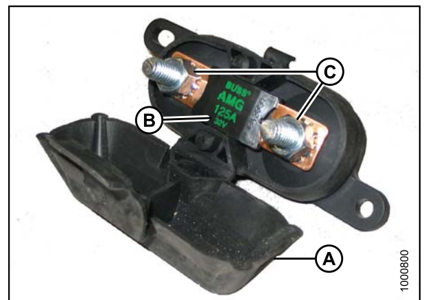
Figure 5.174: 125A Main Fuse
