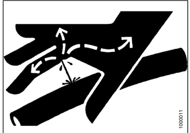
Figure 5.176: Hydraulic Pressure Hazard
