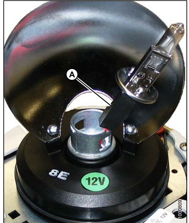
Figure 5.159: Beacon Lamp Assembly
