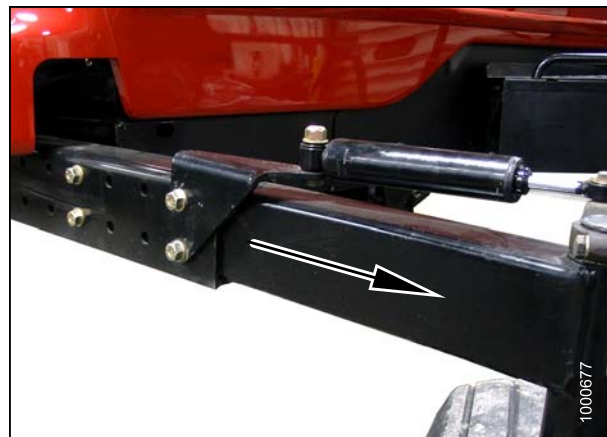
Figure 4.29: Caster Wheel Extensions
