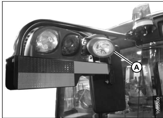
Figure 3.29: HID Auxiliary Lights (Optional)
