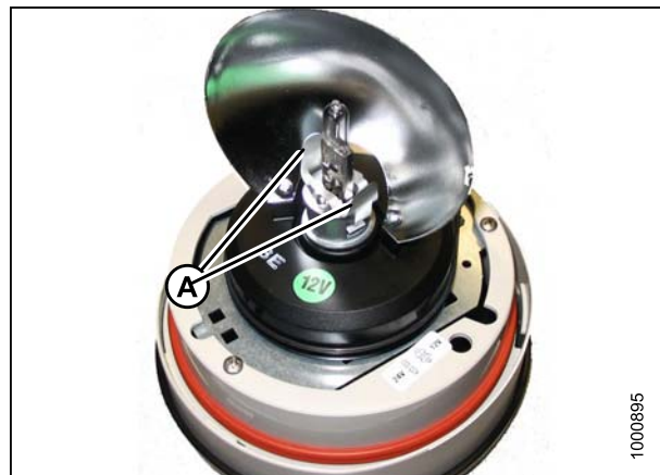
Figure 5.158: Beacon Lamp Assembly
