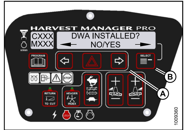
Figure 3.117: M155 DWA Controls
