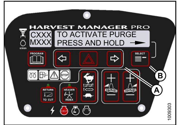
Figure 3.192: M155 Hydraulic Purge
