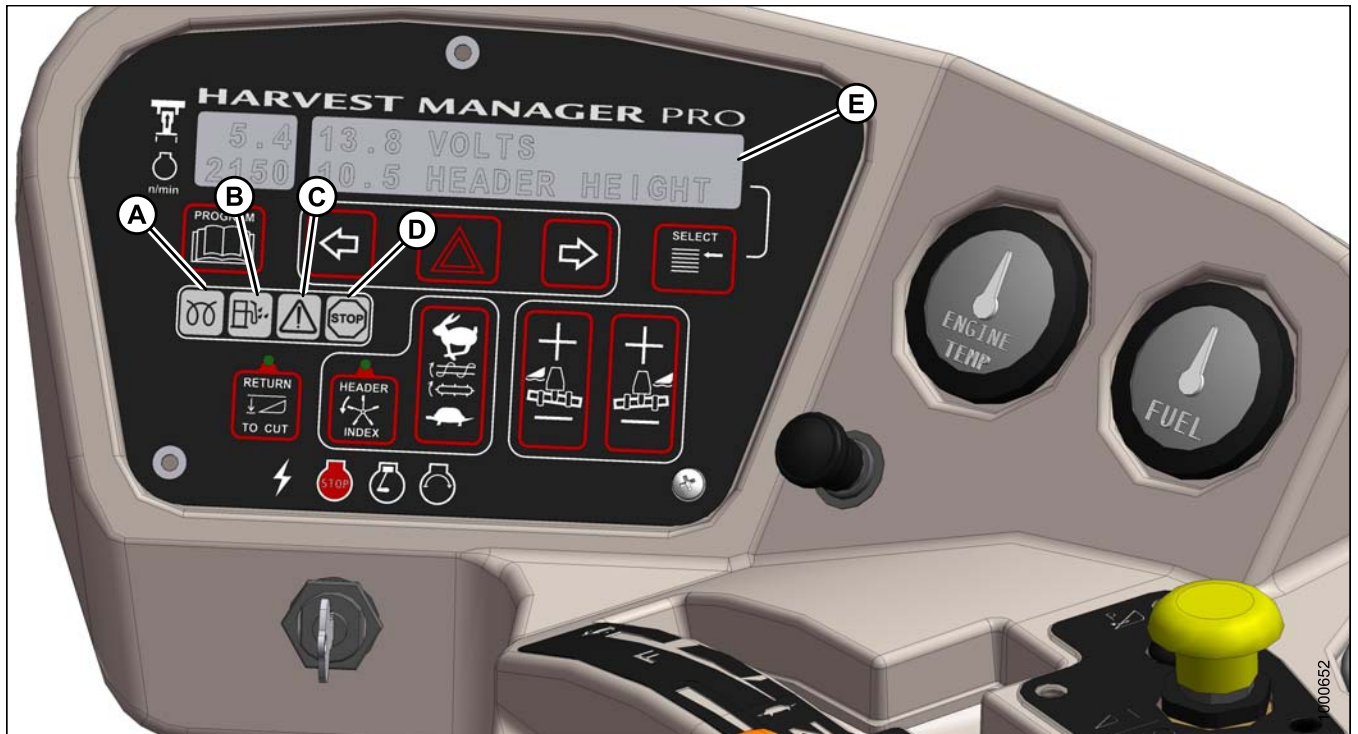
Figure 3.68: CDM Engine Warning Lights
