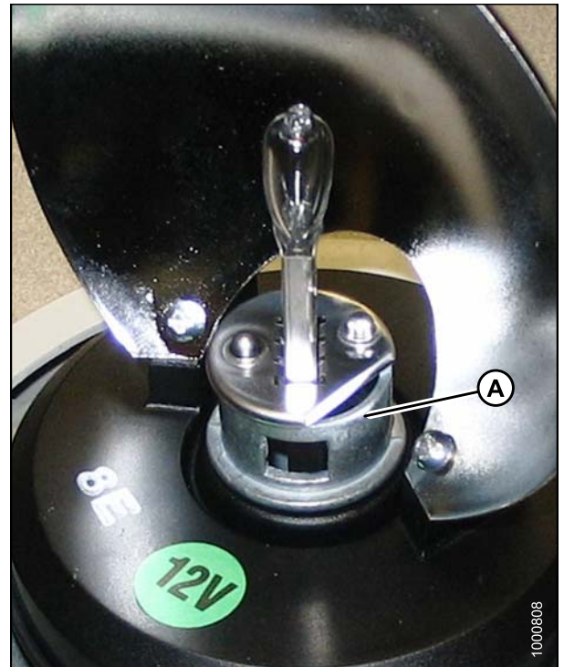
Figure 5.160: Beacon Lamp Assembly
