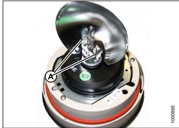
Figure 5.161: Beacon Lamp Assembly
