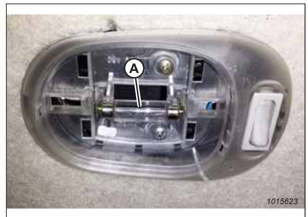
Figure 5.209: Cabin Dome Light with Cover Removed
