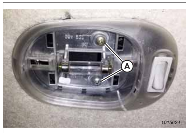
Figure 5.212: Cabin Dome Light with Cover Removed
