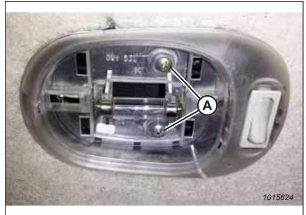
Figure 5.214: Cabin Dome Light with Cover Removed
