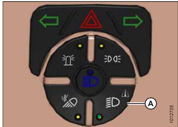
Figure 5.185: Road Light Switch
