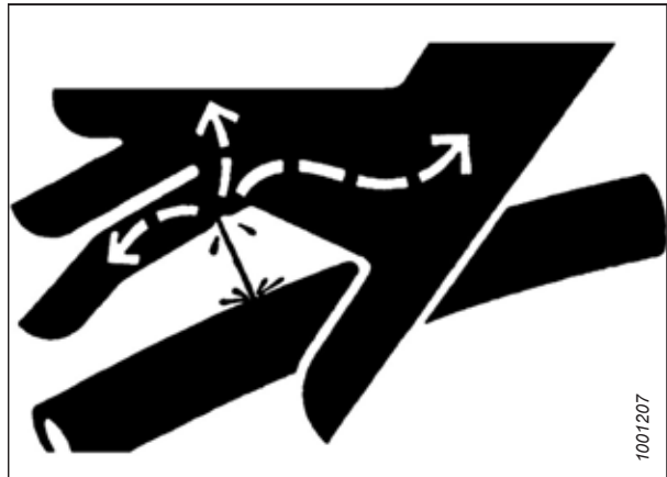
Figure 1.12: Hydraulic Pressure Hazard
