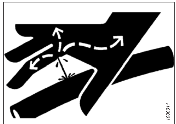
Figure 5.62: Hydraulic Pressure Hazard
