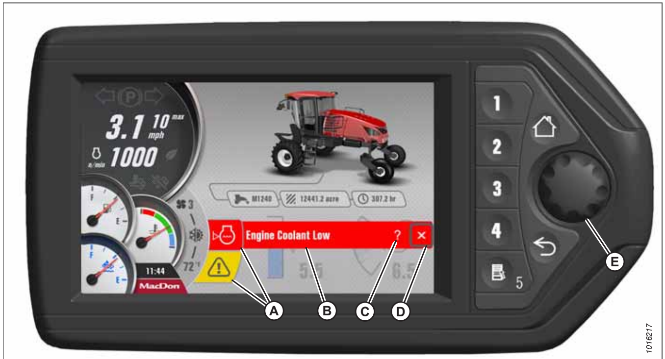
Figure 3.96: HPT Run Screen Displaying Faults
