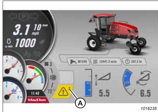
Figure 3.97: Telltale Icon – Multiple Faults Detected
