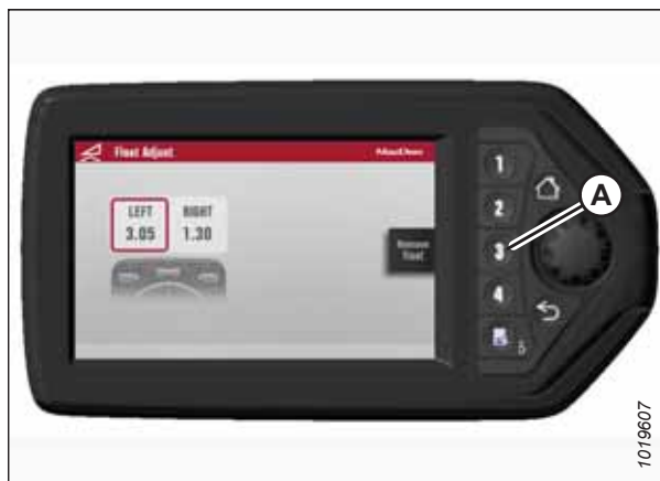
Figure 4.332: HPT Display – Adjusting Float
