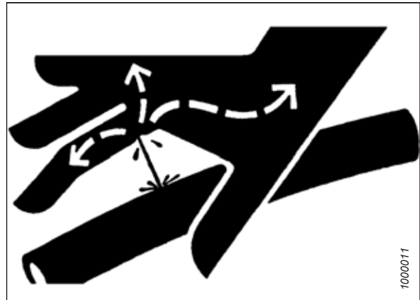
Figure 5.26: Hydraulic Pressure Hazard
