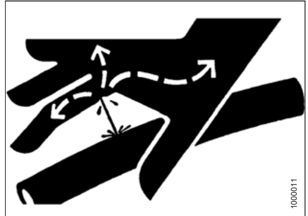
Figure 5.26: Hydraulic Pressure Hazard
