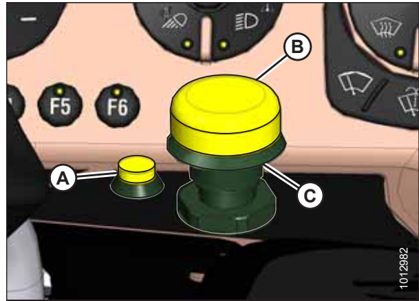
Figure 4.244: Header Drive Controls
