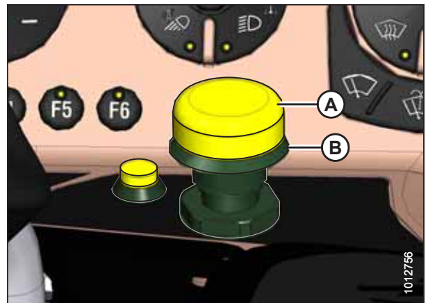
Figure 4.314: Header Engage Switch
