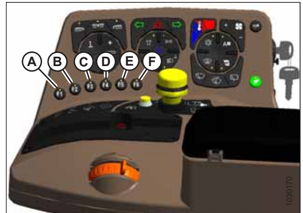
Figure 3.128: Operator's Console Shortcut Buttons
