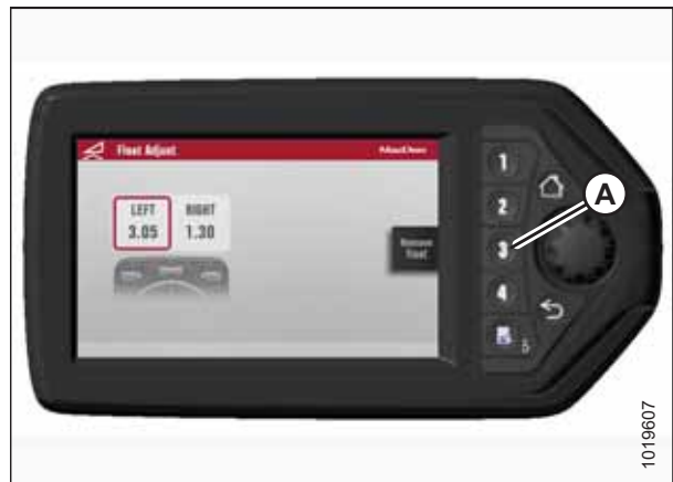
Figure 4.242: HPT Display – Adjusting Float
