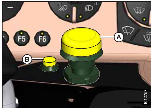
Figure 3.55: Header Drive Controls
