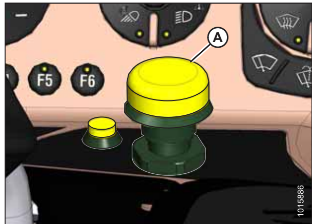
Figure 4.368: Header Engage Switch
