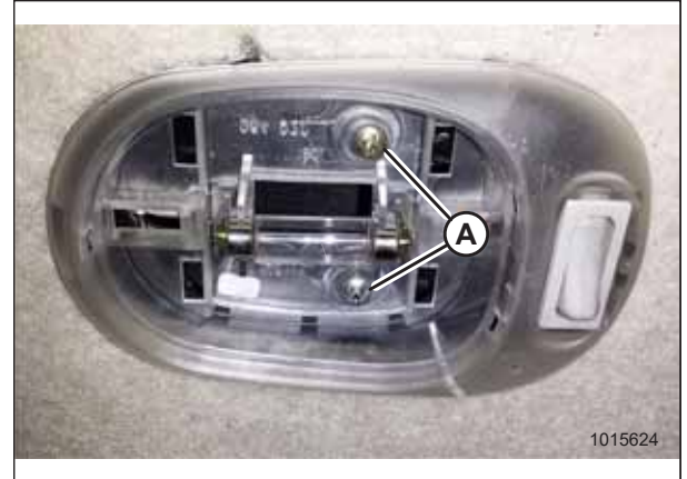
Figure 5.203: Cabin Dome Light with Cover Removed
