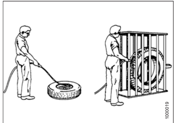
Figure 1.15: Safely Inflating Tire
