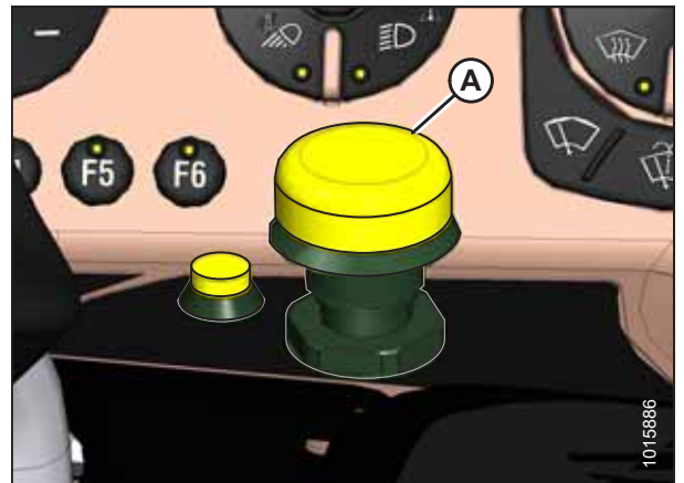
Figure 4.356: Header Engage Switch
