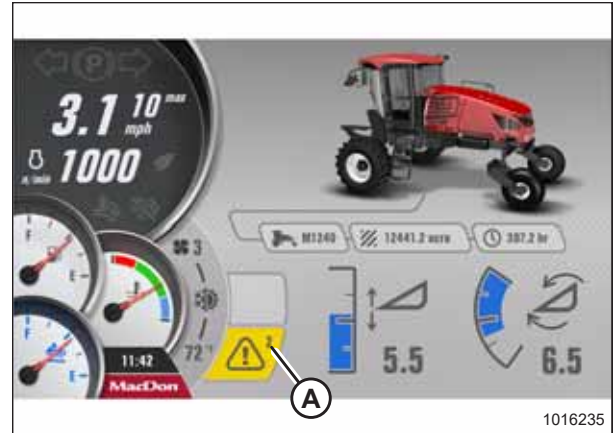
Figure 3.95: Telltale Icon – Multiple Faults Detected
