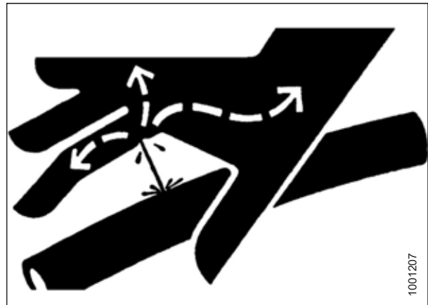
Figure 1.12: Hydraulic Pressure Hazard
