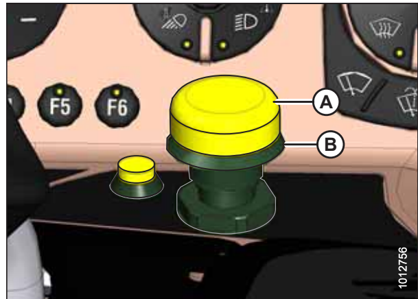
Figure 4.311: Header Engage Switch
