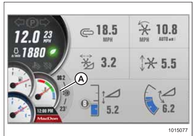
Figure 4.23: HPT Display – Engine Temperature Gauge
