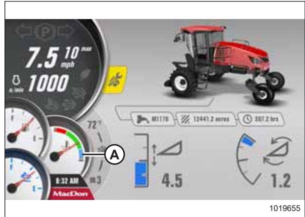
Figure 4.18: HPT No Header Screen
