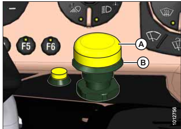
Figure 4.354: Header Engage Switch
