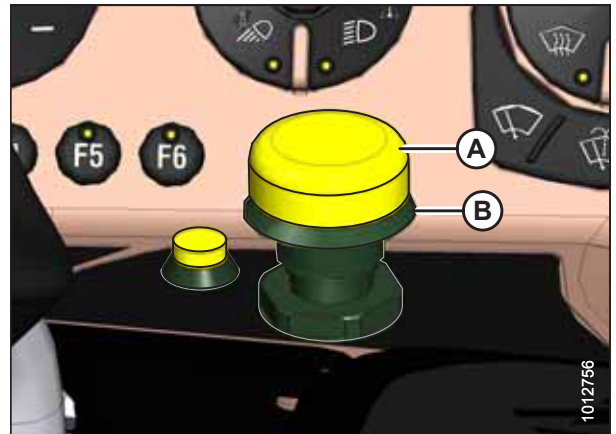
Figure 4.366: Header Engage Switch
