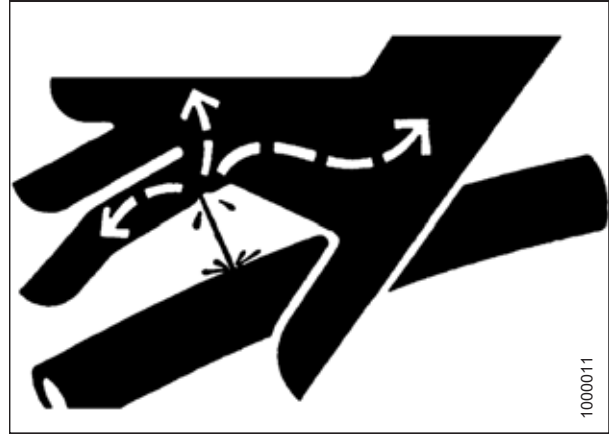
Figure 5.62: Hydraulic Pressure Hazard
