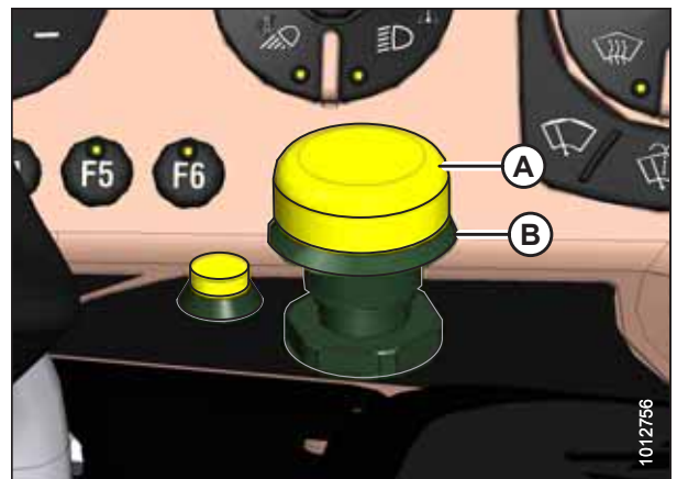
Figure 4.243: Header Engage Switch
