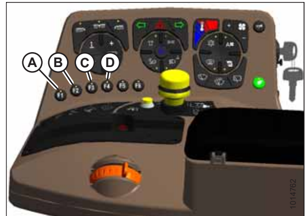
Figure 3.128: Operator's Console Shortcut Buttons
