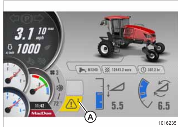
Figure 3.95: Telltale Icon – Multiple Faults Detected
