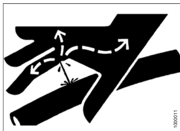
Figure 5.60: Hydraulic Pressure Hazard
