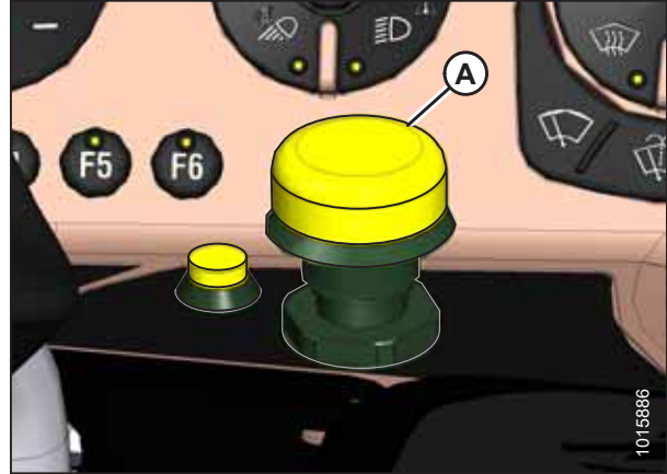
Figure 4.310: Header Engage Switch
