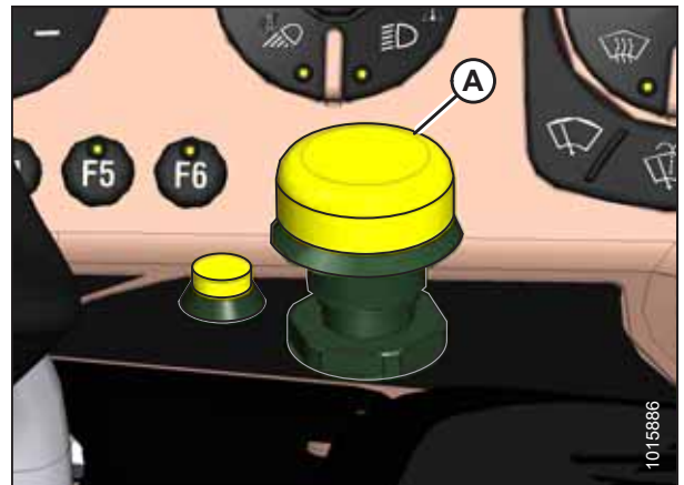
Figure 4.298: Header Engage Switch
