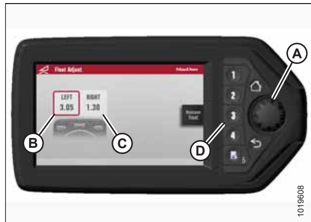
Figure 4.179: HPT Left and Right Float Settings
