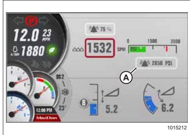
Figure 4.248: Adjusting Knife Alarm Pressure
