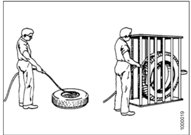
Figure 1.15: Safely Inflating Tire
