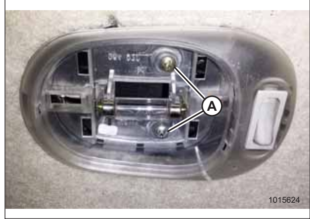
Figure 5.196: Cabin Dome Light with Cover Removed
