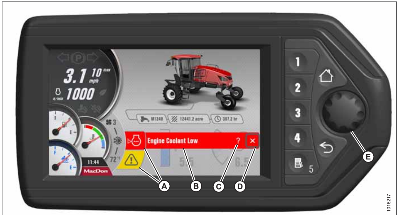
Figure 3.94: HPT Run Screen Displaying Faults
