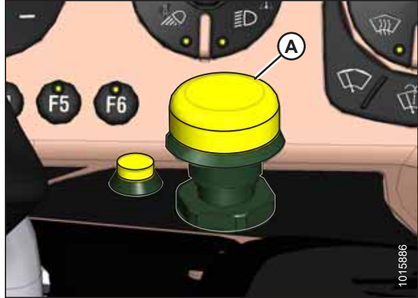
Figure 4.258: Header Engage Switch
