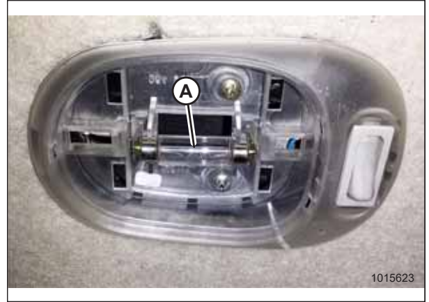
Figure 5.193: Cabin Dome Light with Cover Removed
