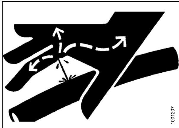
Figure 1.12: Hydraulic Pressure Hazard
