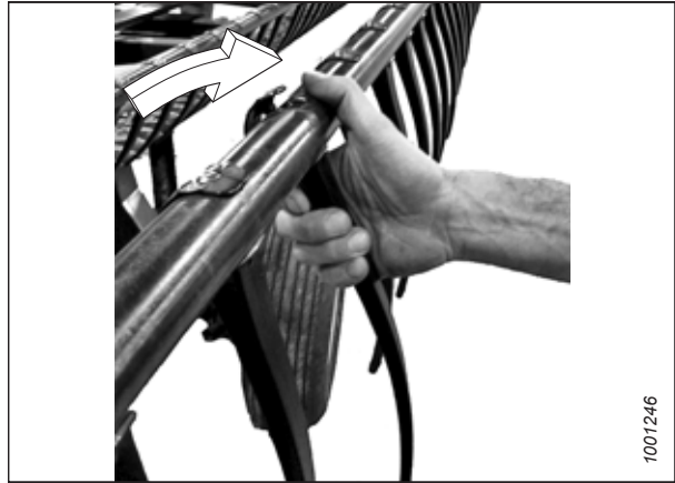
Figure 4.297: Installing Plastic Finger
