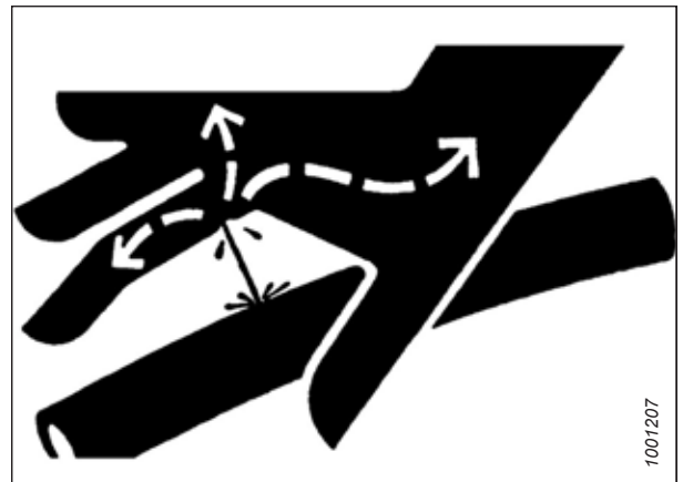
Figure 4.1: Hydraulic Pressure Hazard
