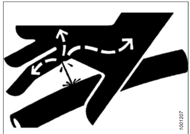
Figure 1.12: Hydraulic Pressure Hazard
