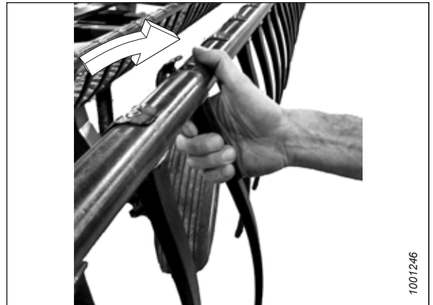
Figure 4.296: Installing Plastic Finger
