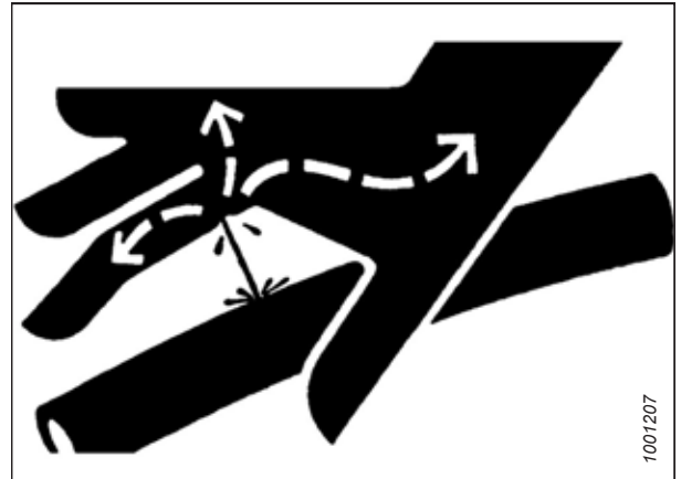
Figure 4.1: Hydraulic Pressure Hazard
