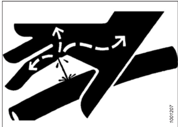
Figure 1.12: Hydraulic Pressure Hazard
