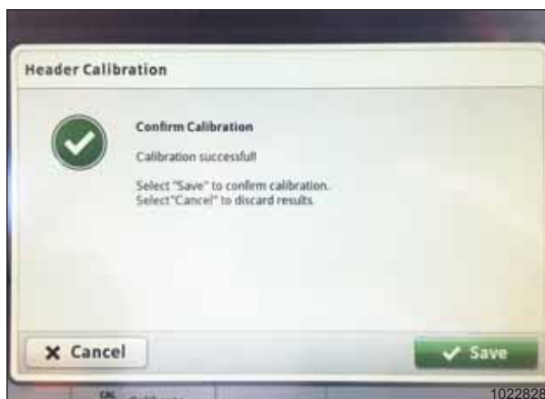
Figure 3.495: John Deere S7 ekraan – heedri kalibreerimine
