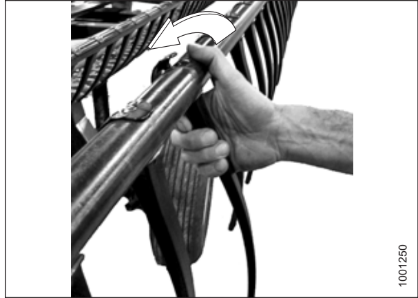
Figure 5.314: Removing Plastic Finger
