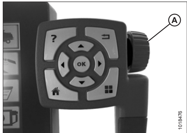
Figure 3.402: Adjustment Wheel on Right Side of Tyton Terminal
