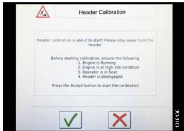
Figure 3.213: Header Calibration Warning
