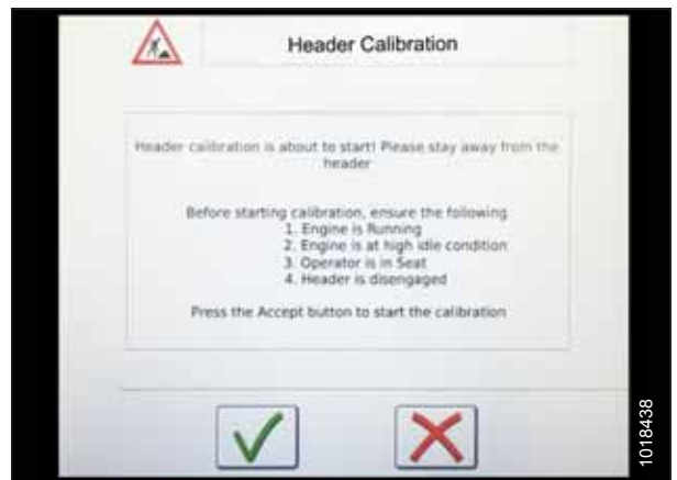
Figure 3.393: Header Calibration Warning
