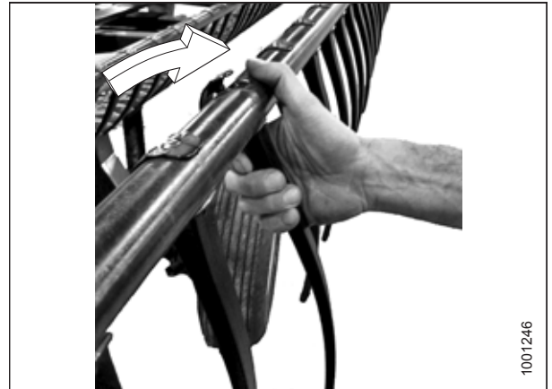
Figure 5.315: Installing Plastic Finger
