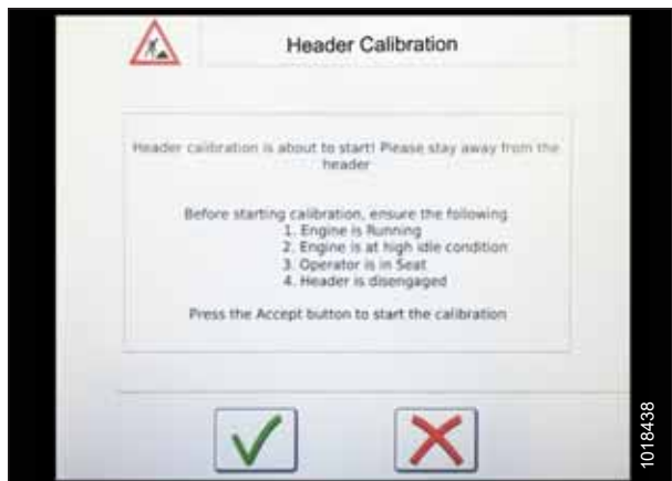
Figure 3.365: Header Calibration Warning
