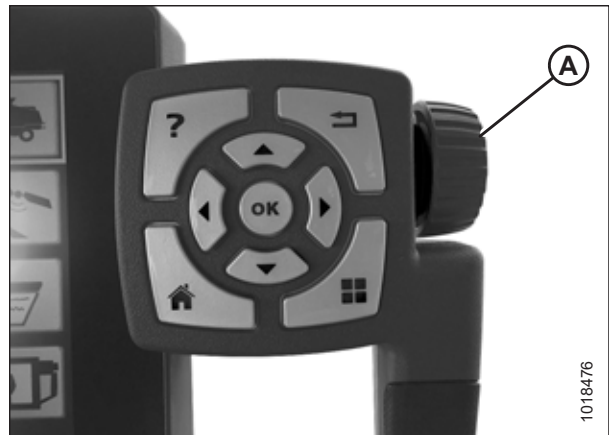
Figure 3.193: Adjustment Wheel on Right of Tyton Terminal
