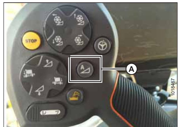
Figure 3.190: AHHC on Control Handle
