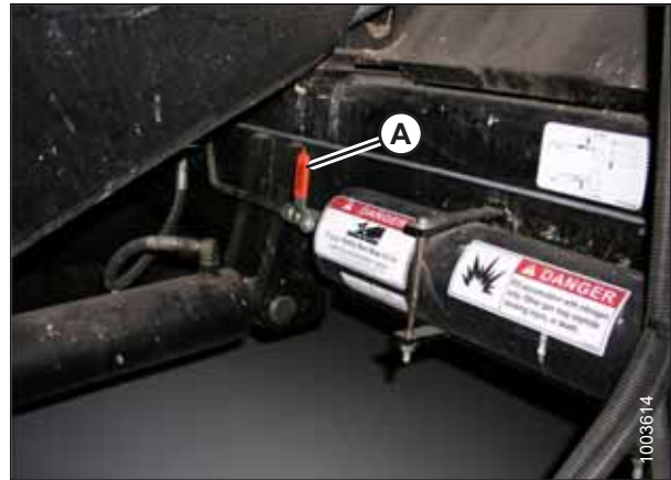
Figure 3.334: Combine Accumulator ON/OFF Switch
