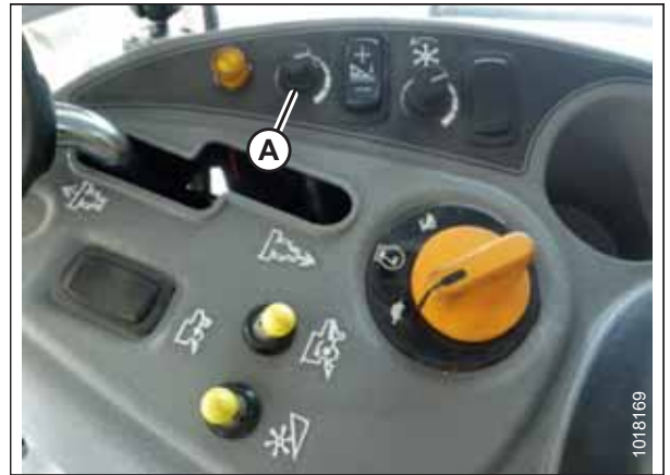
Figure 3.258: Height Adjustment Knob on the Combine Control Console
