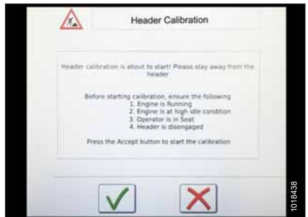
Figure 3.184: Header Calibration Warning
