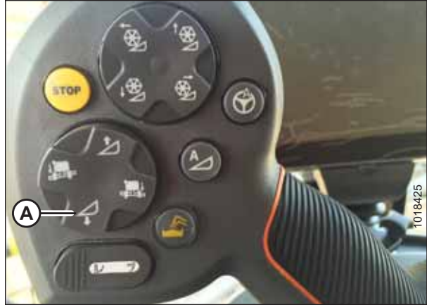
Figure 3.363: Header Down Switch
