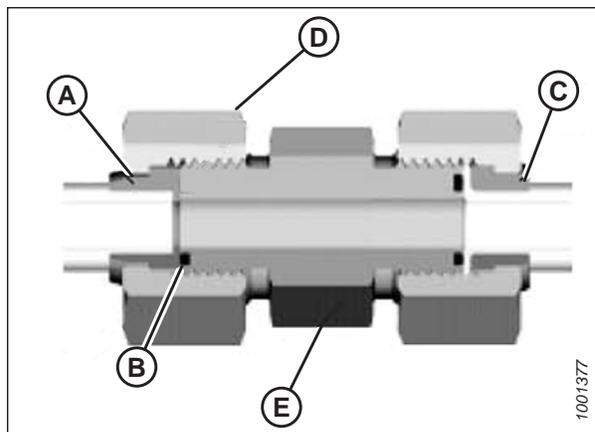
Figure 7.10: Raccord hydraulique
