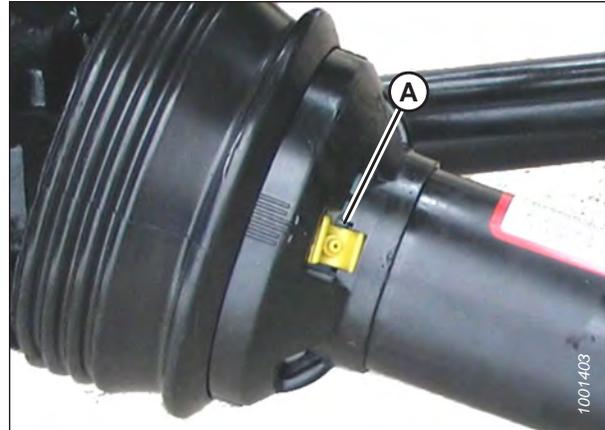
Figure 4.60: Protection de transmission
