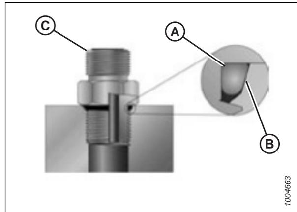
**Figure 7.8: Raccord hydraulique**
