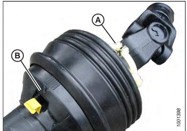
Figure 4.57: Protection de transmission
