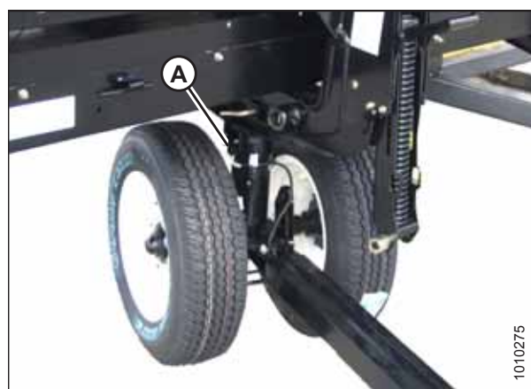
Figure 3.89: Raccordement du faisceau
