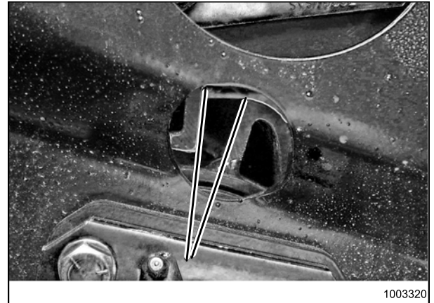
Figure 8.230: Conditioner Bars Not in Time (Right Side)
