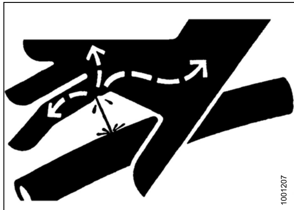
Figure 1.12: Hydraulic Pressure Hazard
