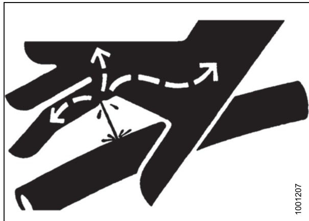
Figure 1.12: Hydraulic Pressure Hazard
