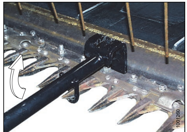
Figure 6.33: Guard Tip – Upward Adjustment
