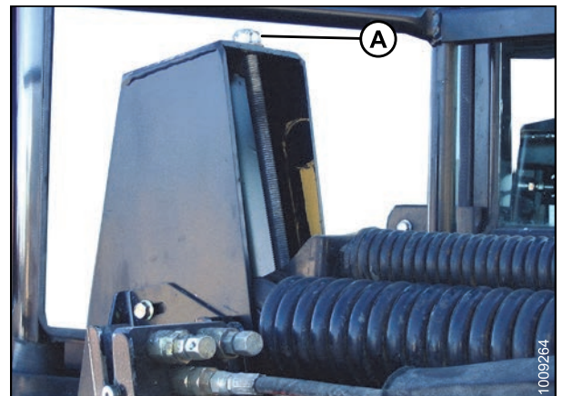
Figure 4.104: Drawbolt – Top of Windrower Wheel Leg Member Shown
