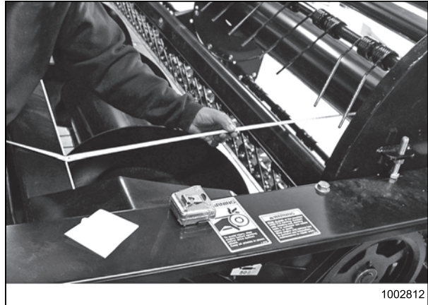
Figure 3.76: Reel Fore-Aft Offset
