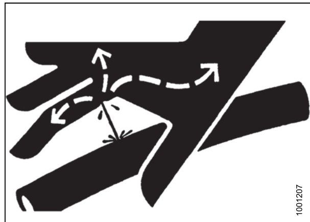
Figure 6.19: Hydraulic Pressure Hazard
