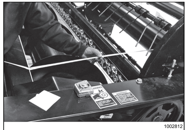
Figure 4.88: Reel Fore-Aft Offset
