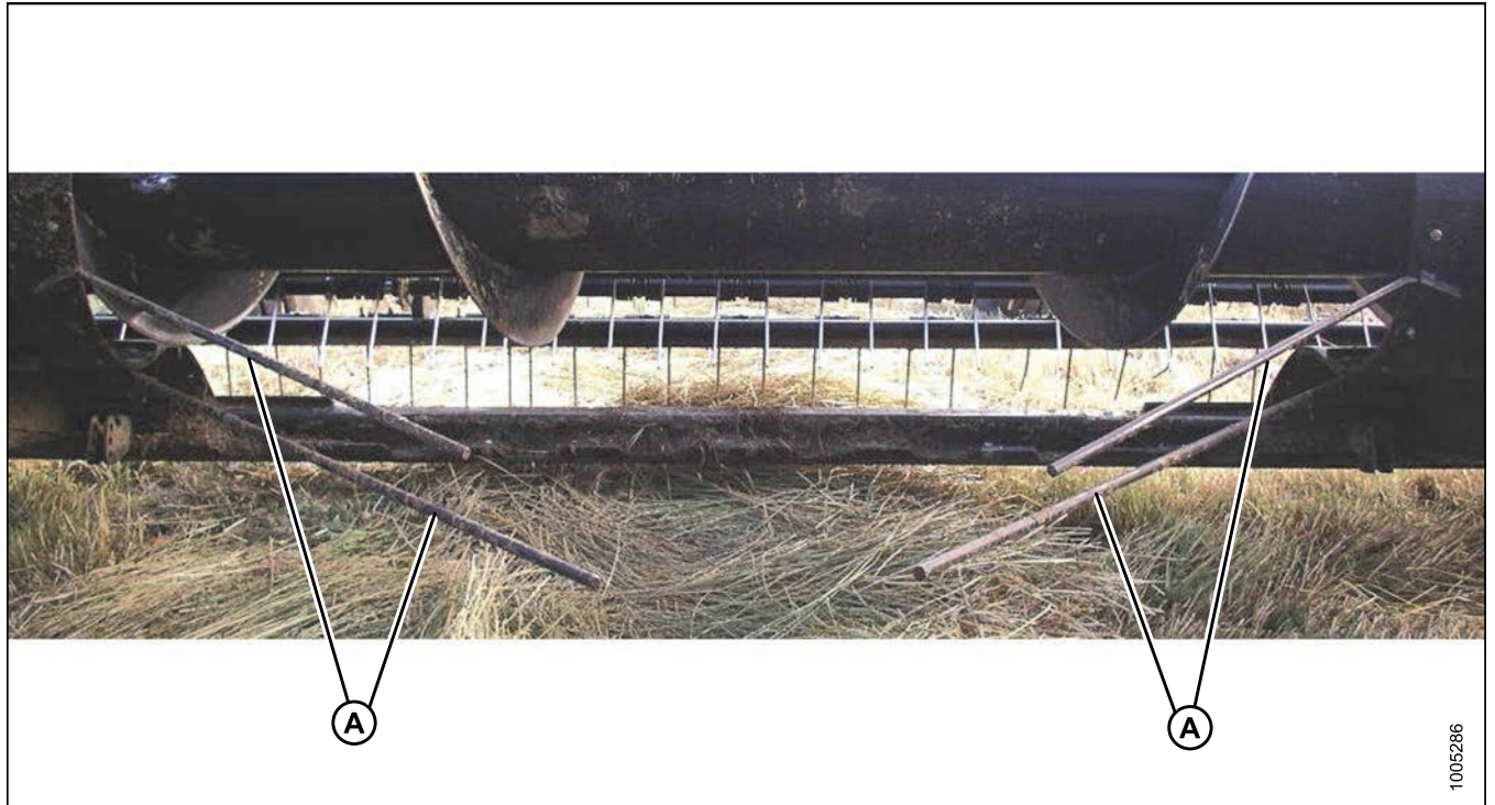
Figure 4.119: Windrow Forming Rods
