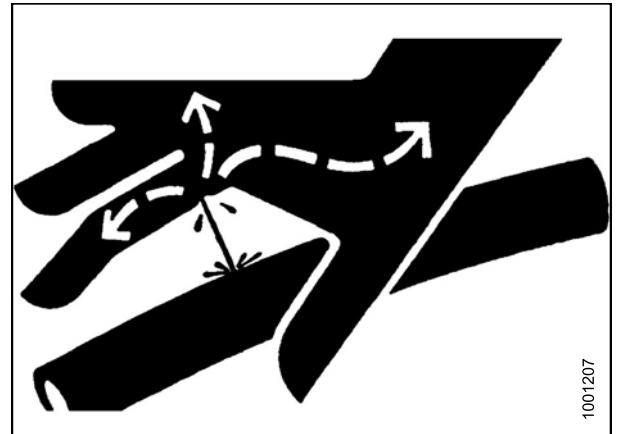
Figure 4.10: Hydraulic Pressure Hazard
