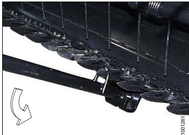
Figure 4.23: Guard Tip – Downward Adjustment
