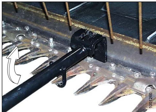
Figure 4.24: Guard Tip – Upward Adjustment
