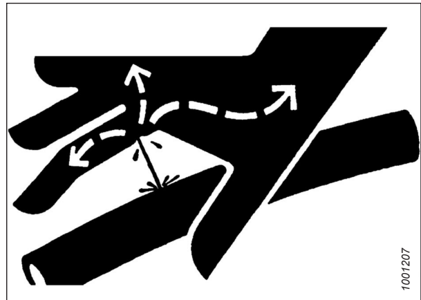
Figure 4.15: Hydraulic Pressure Hazard
