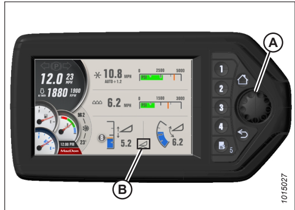
Figure 3.144: HPT Run Screen
