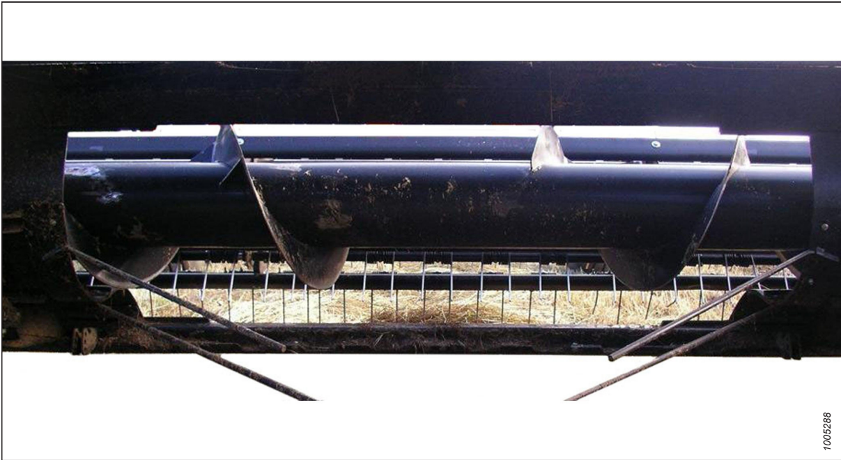
Figure 3.164: Grass Seed Auger
