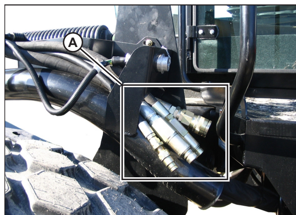
Figure 3.26: Header Drive Hoses
