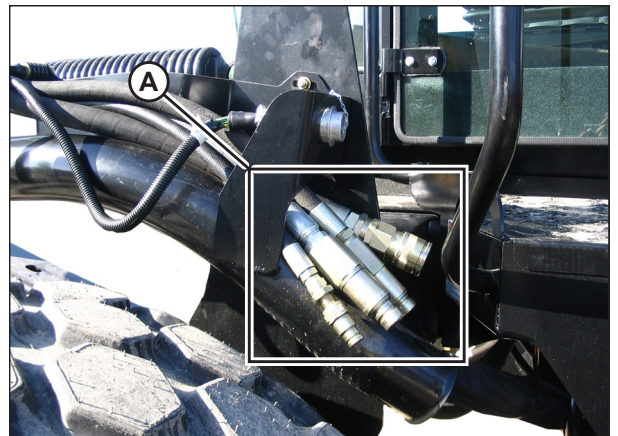
Figure 3.40: Header Drive Hoses
