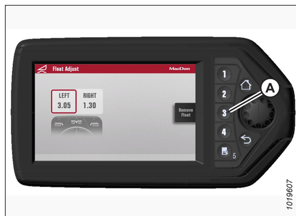
Figure 3.147: HPT Display – Adjusting Float
