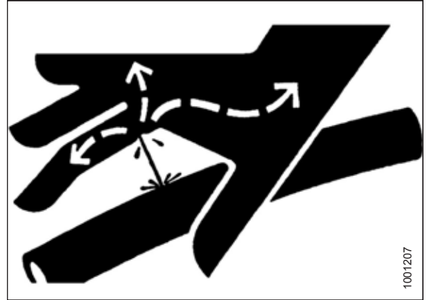
Figure 4.10: Hydraulic Pressure Hazard
