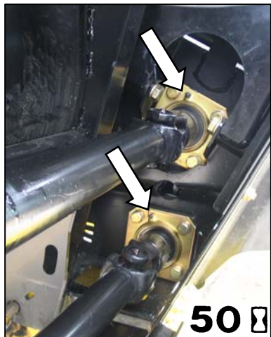
ROLL SHAFT BEARINGS (2 PLCS)
