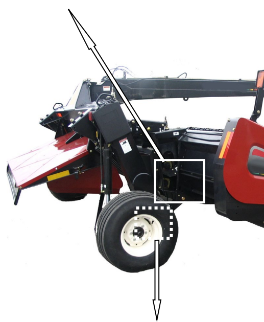
LIFT LINKAGE (2 PLCS) – BOTH SIDES
