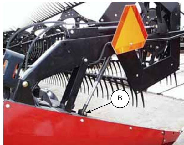
REEL LIFT CYLINDERS WORKING POSITION
