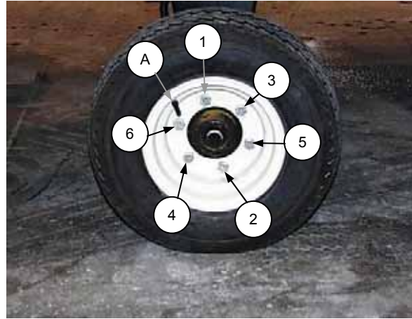
BOLT TIGHTENING SEQUENCE
