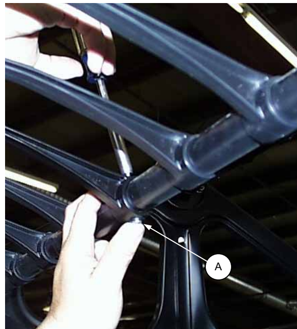
INSTALLING PLASTIC FINGERS
