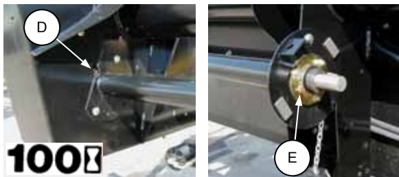
SICKLE DRIVE SHAFT SUPPORT BEARINGS
