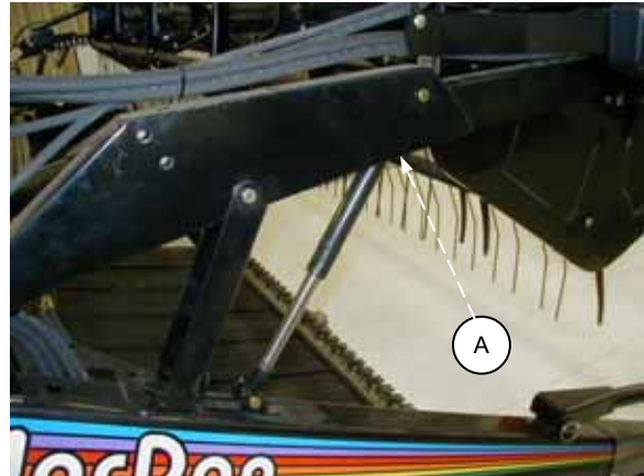
REEL LIFT CYLINDER BLEED SCREW
