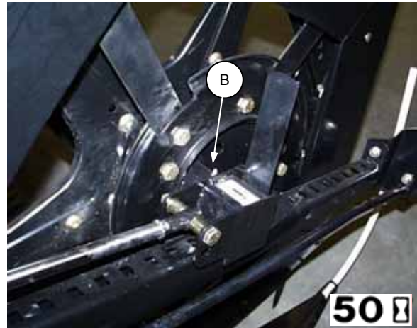
REEL SUPPORT BUSHINGS – R/H SPLIT PICK-UP REEL HEADER
