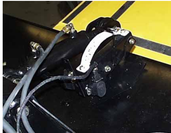
USE FLOAT OPTIMIZER GAUGE TO BALANCE WINGS
