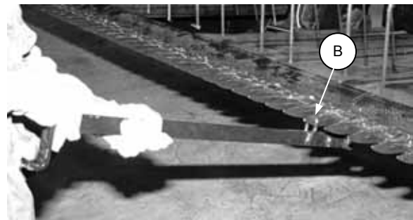
BENDING GUARD TIPS DOWN
