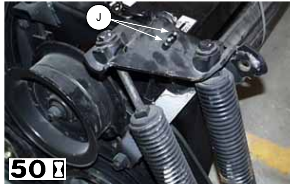
HAY CONDITIONER ROLL BEARINGS (BOTH SIDES)
