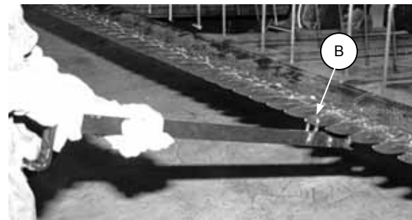
BENDING GUARD TIPS DOWN
