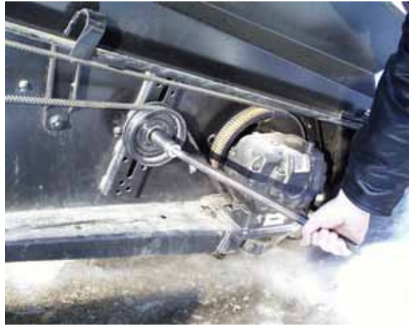
DOUBLE SICKLE IDLER ALIGNMENT
