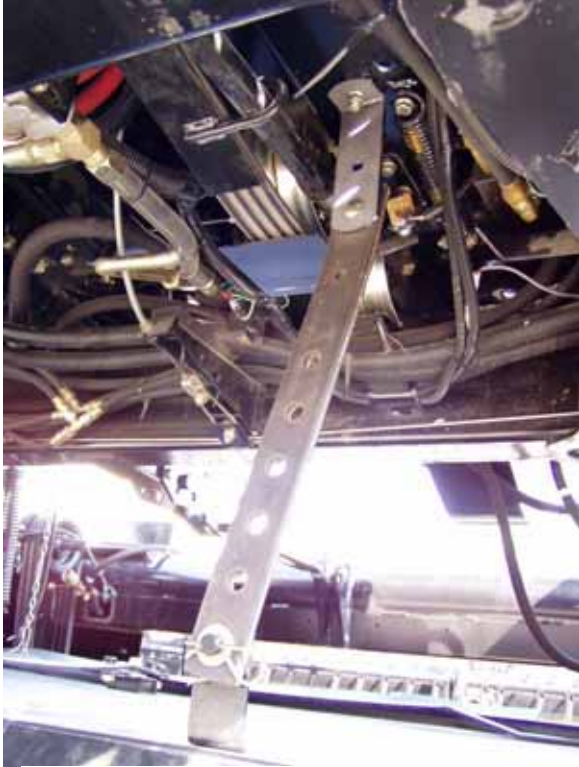
XX52 & XX52i FORMING SHIELD SUPPORT STRAP
