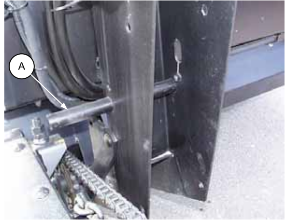
INSTALL CONDITIONER STOP ROD
