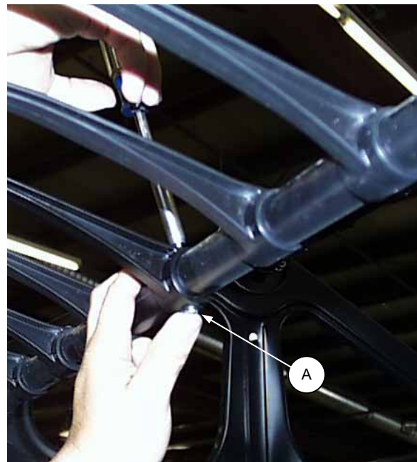
INSTALLING PLASTIC FINGERS
