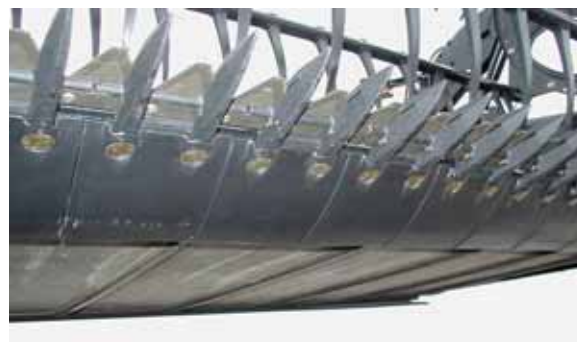
CUTTERBAR POLY WEAR STRIPS
