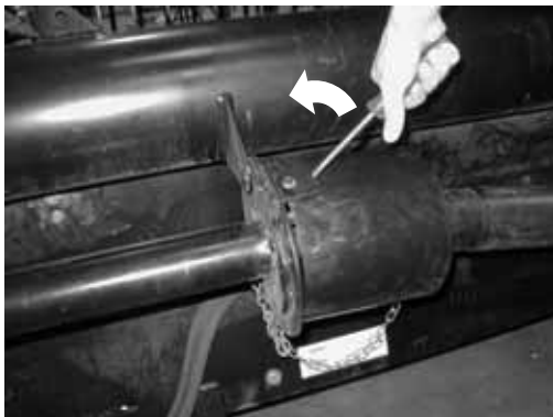
REMOVING DRIVELINE SHIELD
