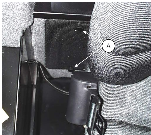
REMOVE FOR ACCESS TO RETURN AIR FILTER
