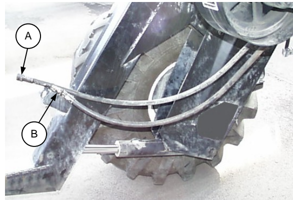
HYDRAULIC CONNECTIONS - R/H SIDE
