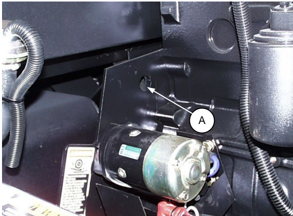
BARRING TOOL ACCESS HOLE
