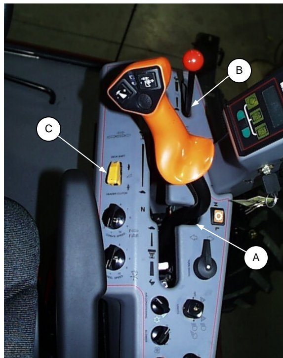
CONTROL LEVERS - STOPPING
