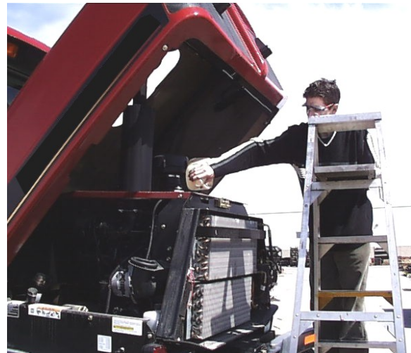
USE LADDER TO ACCESS RADIATOR
