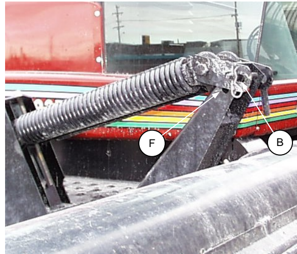
ATTACH FLOAT SPRINGS
