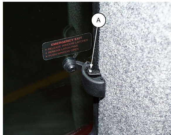
R/H SIDE WINDOW - EMERGENCY EXIT
