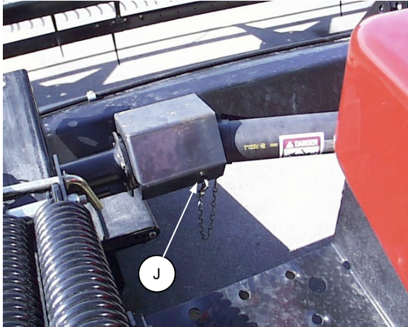
CONNECT DRIVELINE – 962/963 HEADER
