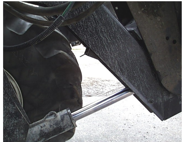
LIFT CYLINDER STOP - STORAGE
