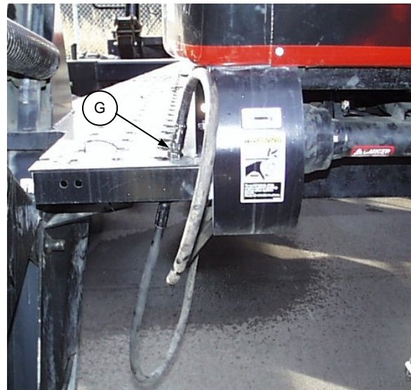
TRACTOR REEL DRIVE HOSES - STORAGE
