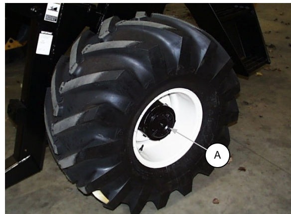
DISENGAGE FINAL DRIVES
