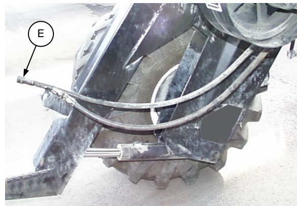
ATTACH PRESSURE GAUGE
