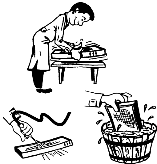
CLEANING AIR FILTER
