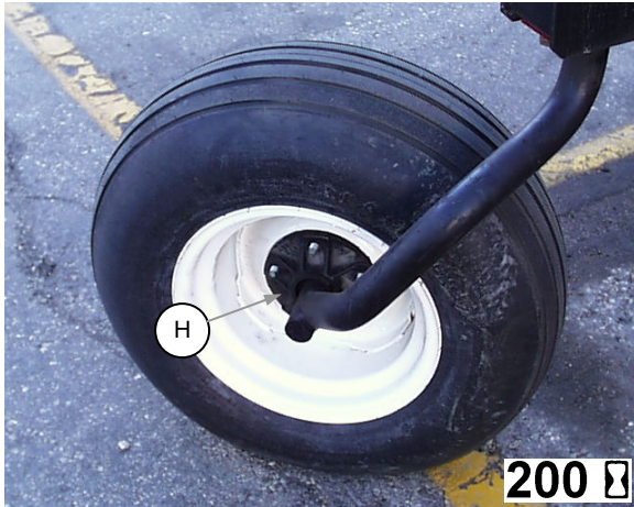
CASTER WHEEL HUB BEARINGS (H) TWO FITTINGS
