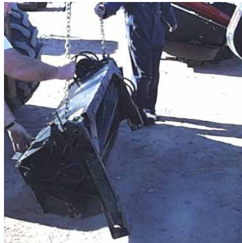
ATTACH CHAIN AT SIDE FRAMES OR U-BOLT
