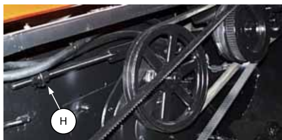
LOOSEN AUGER DRIVE BELT FIRST
