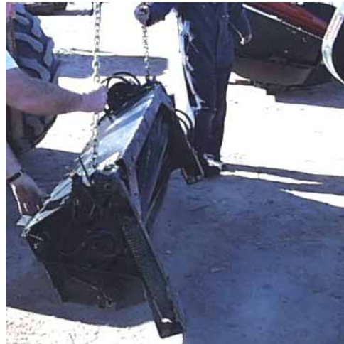
ATTACH CHAIN AT SIDE FRAMES OR U-BOLT
