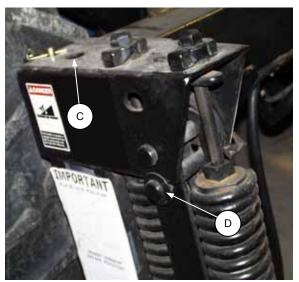
R/H FLOAT LOCK-OUT PIN - ENGAGED
