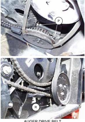
AUGER DRIVE BELT TENSION ADJUSTMENT
