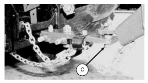
CHECK HITCH PIN LOCK NUT
