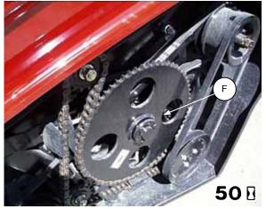
AUGER SHAFT BEARING - LEFT SIDE Form # 147008
