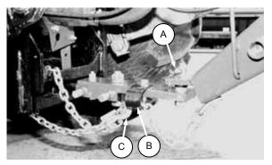
SECURE HITCH PIN AND CHAIN
