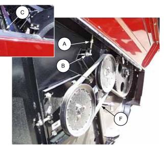
REEL DRIVE BELT TENSION ADJUSTMENT
