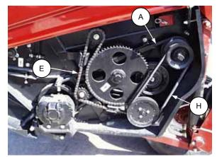
CHECK SICKLE DRIVE BELT AND AUGER DRIVE BELT & CHAIN TENSION
