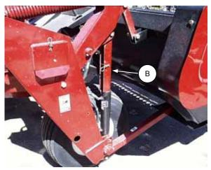
LIFT CYLINDER STOPS - ENGAGED
