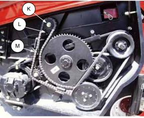
AUGER DRIVE CHAIN TENSION ADJUSTMENT
