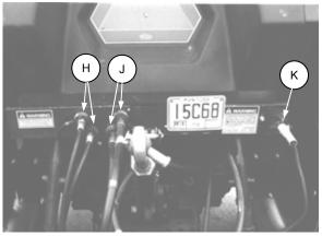
CONNECT REMOTE HYDRAULICS AND ELECTRICAL
