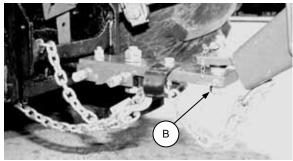
CHECK HITCH PIN LOCK NUT
