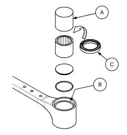
NEEDLE BEARING INSTALLATION
