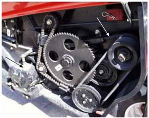
CHECK SICKLE DRIVE BELT TENSION, AND DRIVE BOX LUBRICANT
