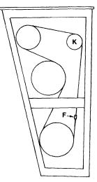
CONNECT CHAIN AND INSTALL TENSIONER SPROCKET
