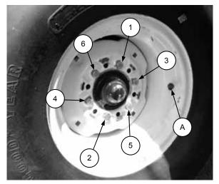
WHEEL BOLT TIGHTENING SEQUENCE
