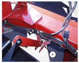
ADJUST LINK TO CENTER OF SLOT
