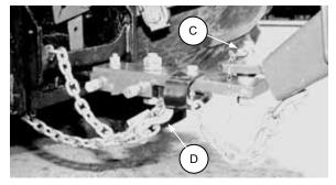
REMOVE HITCH PIN LOCK AND CHAIN
