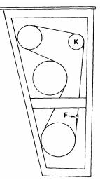
CONNECT CHAIN AND INSTALL TENSIONER SPROCKET
