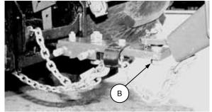
CHECK HITCH PIN LOCK NUT
