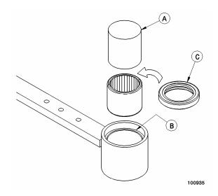
NEEDLE BEARING INSTALLATION
