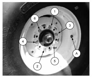
WHEEL BOLT TIGHTENING SEQUENCE
