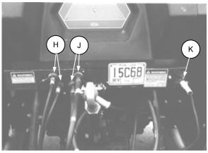
CONNECT REMOTE HYDRAULICS AND ELECTRICAL
