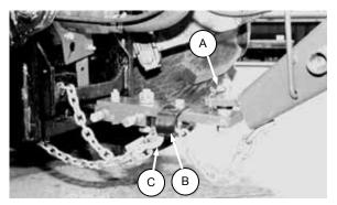
SECURE HITCH PIN AND CHAIN
