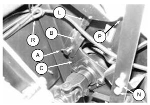
REMOVE ROLL GAP ADJUSTMENT ROD
