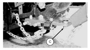
CHECK HITCH PIN LOCK NUT
