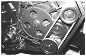
CHECK SICKLE DRIVE BELT TENSION, AND DRIVE BOX LUBRICANT
