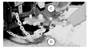
REMOVE HITCH PIN LOCK AND CHAIN
