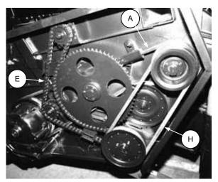
CHECK SICKLE DRIVE BELT AND AUGER DRIVE BELT & CHAIN TENSION
