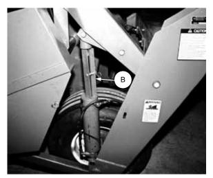
LIFT CYLINDER STOPS - ENGAGED
