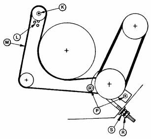
AUGER DRIVE CHAIN AND BELT **TENSION ADJUSTMENT**
