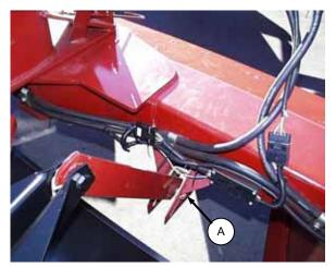
ADJUST LINK TO CENTER OF SLOT
