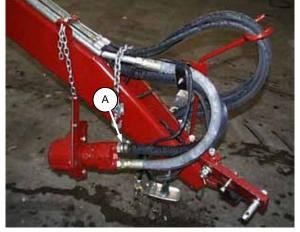
DRAIN RESERVOIR AT PUMP SUPPLY HOSE
