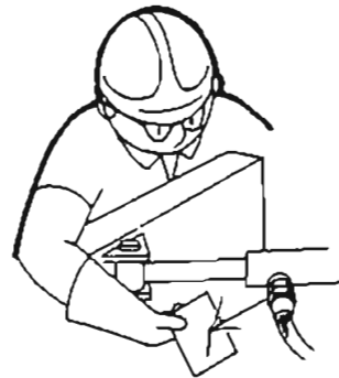
CHECK PROPERLY FOR LEAKS
