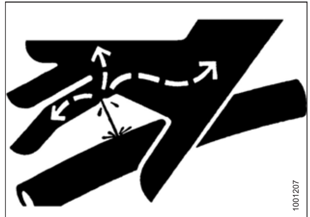
Figure 4.211: Hydraulic Pressure Hazard
