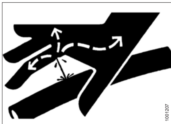
Figure 1.9: Hydraulic Pressure Hazard
