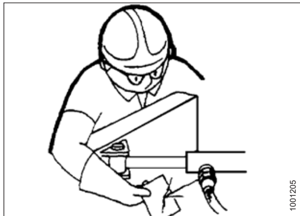
Figure 1.8: Testing for Hydraulic Leaks
