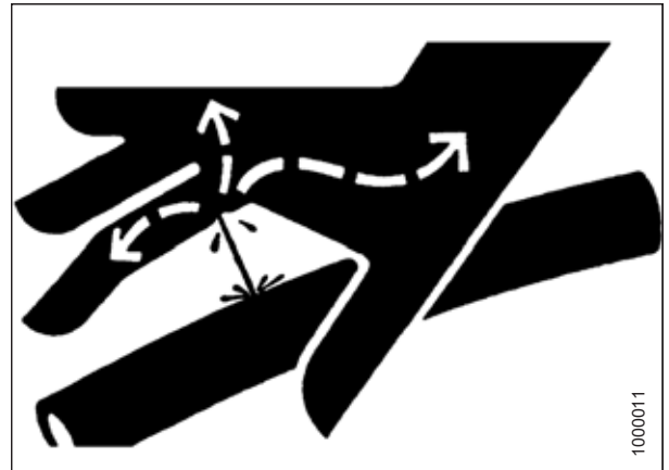
Figure 6.187: Hydraulic Pressure Hazard
