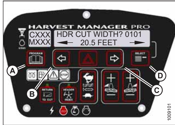
Figure 3.102: Header Cut Width
