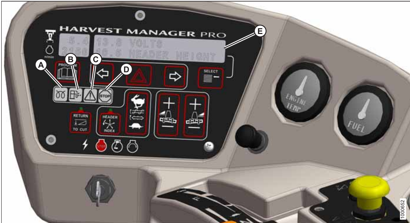
Figure 3.61: CDM Engine Warning Lights
