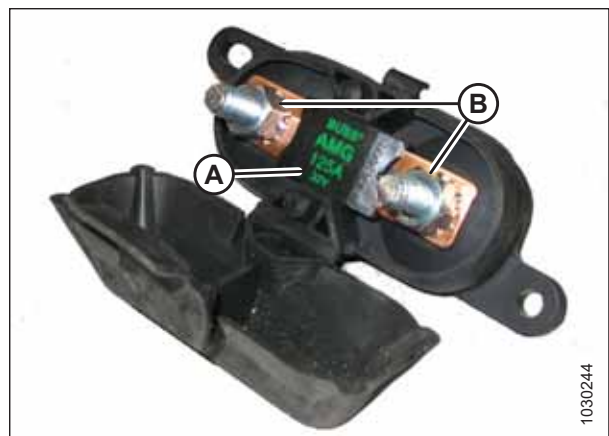
Figure 6.185: 125A Main Fuse
