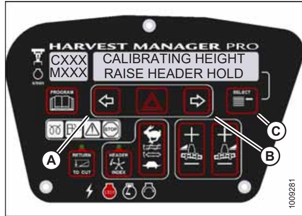
Figure 3.146: Header Height Calibration
