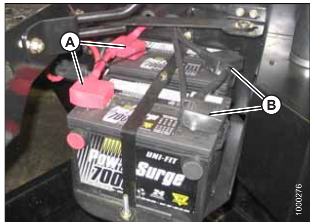
Figure 6.130: Battery Terminal Location
