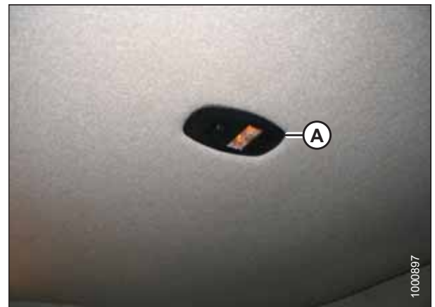
Figure 6.178: Ambient Light Fixture
