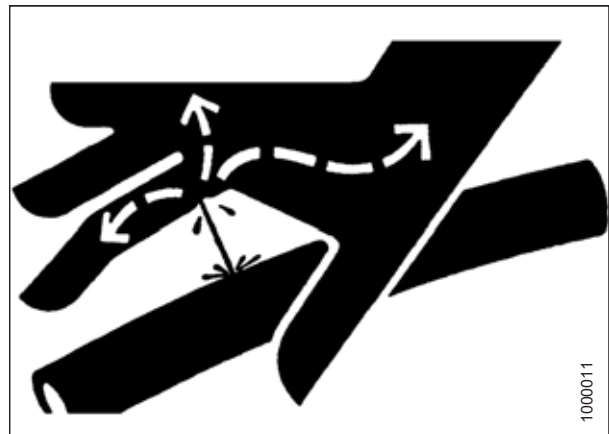
Figure 6.200: Hydraulic Pressure Hazard
