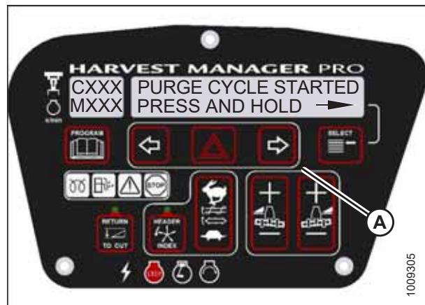
Figure 3.217: Hydraulic Purge Cycle
