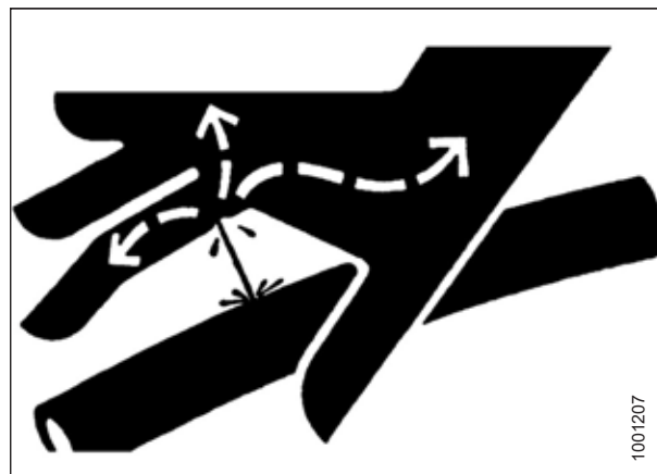
Figure 1.12: Hydraulic Pressure Hazard
