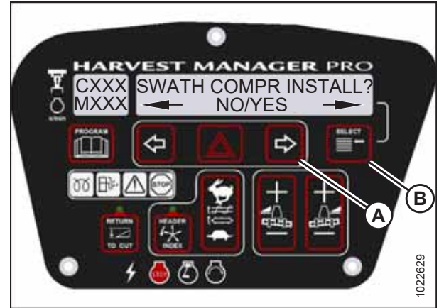
Figure 3.104: Swath Compressor Controls
