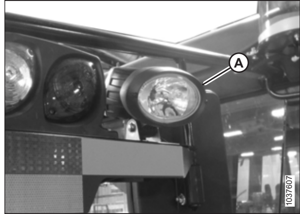
Figure 6.162: New HID Lamp in Place
