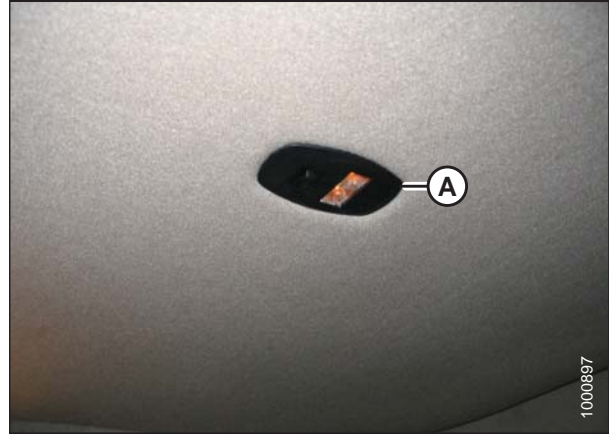
Figure 5.181: Ambient Light Fixture
