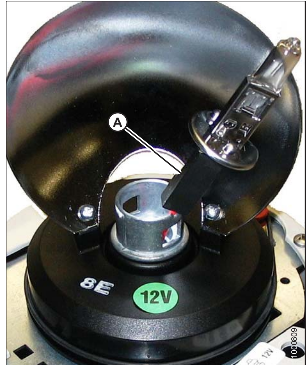
Figure 5.175: Beacon Lamp Assembly
