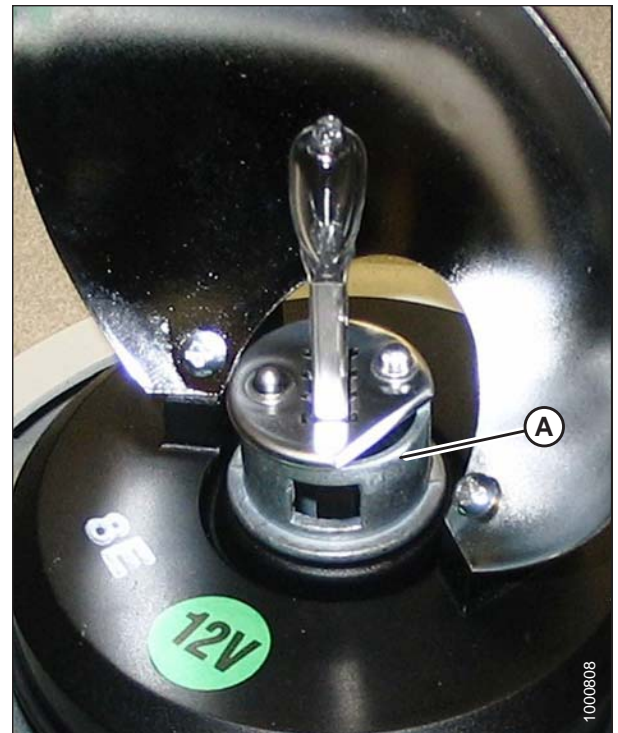
Figure 5.176: Beacon Lamp Assembly
