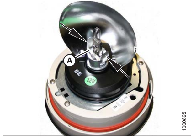
Figure 5.177: Beacon Lamp Assembly
