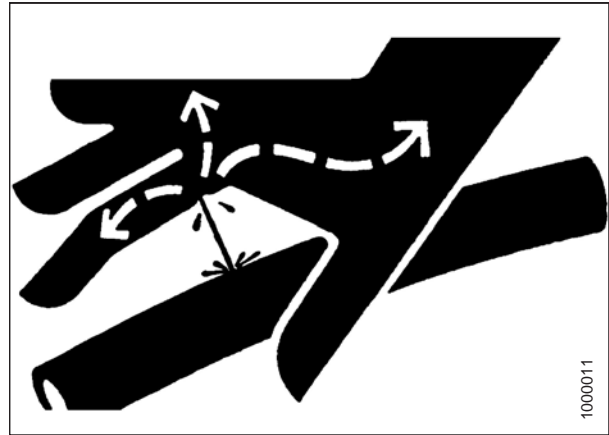
Figure 5.195: Hydraulic Pressure Hazard
