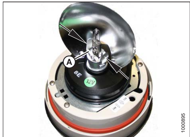
Figure 5.174: Beacon Lamp Assembly
