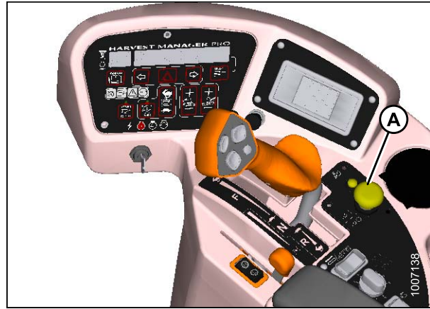
Figure 4.32: Header Drive Switch
