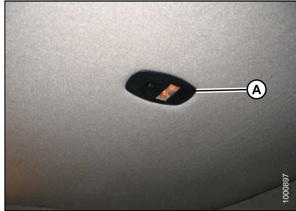
Figure 5.177: Ambient Light Fixture
