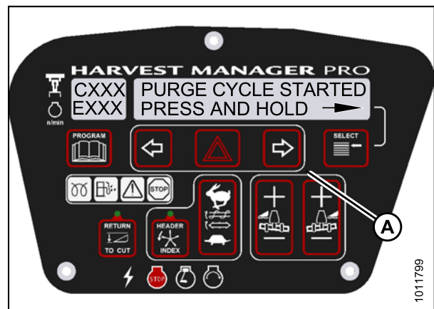
Figure 3.200: Hydraulic Purge Cycle
