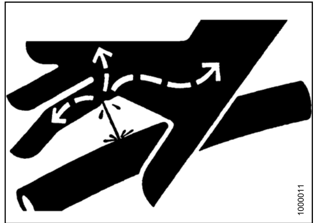
Figure 5.208: Hydraulic Pressure Hazard
