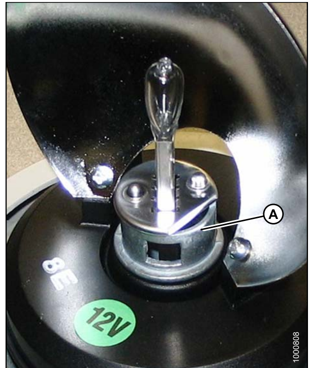
Figure 5.172: Beacon Lamp Assembly
