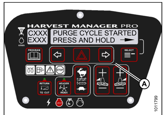
Figure 3.200: Hydraulic Purge Cycle
