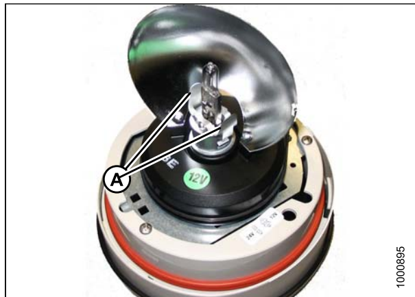
Figure 5.170: Beacon Lamp Assembly
