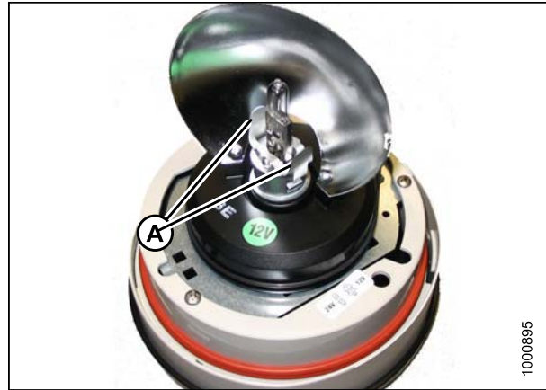
Figure 5.173: Beacon Lamp Assembly
