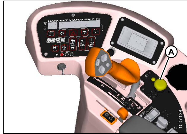
Figure 4.34: Header Drive Switch
