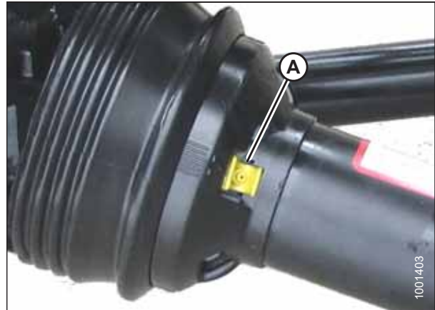
Figure 4.60: Protection de transmission
