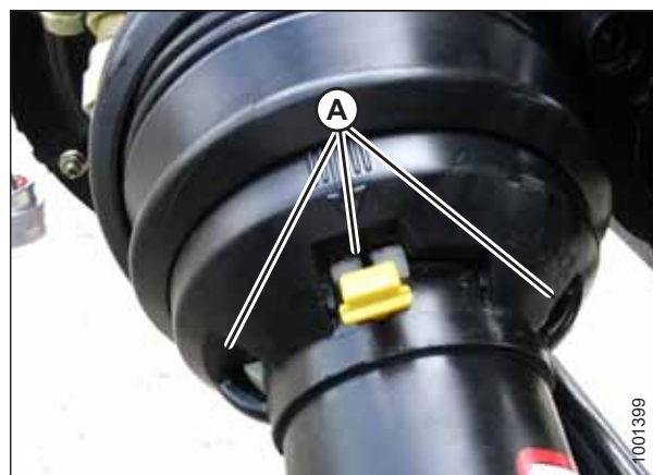
Figure 4.58: Protection de transmission
