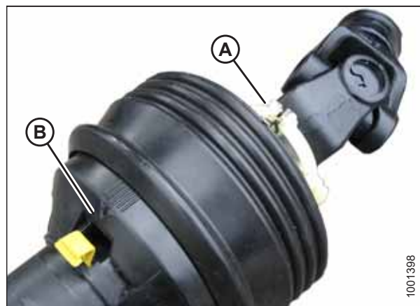
Figure 4.57: Protection de transmission
