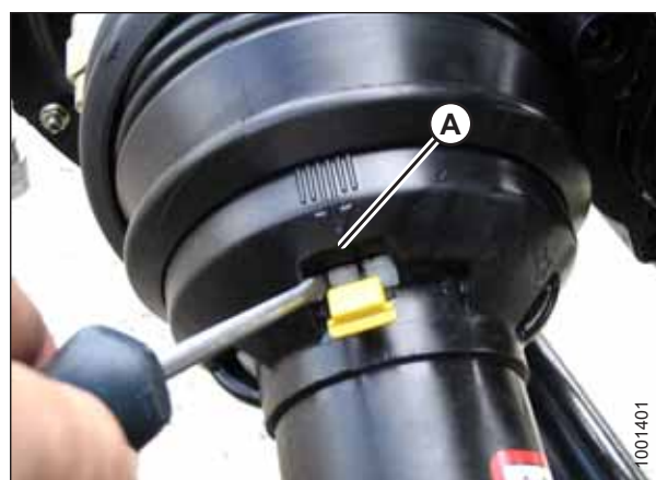
Figure 4.59: Protection de transmission
