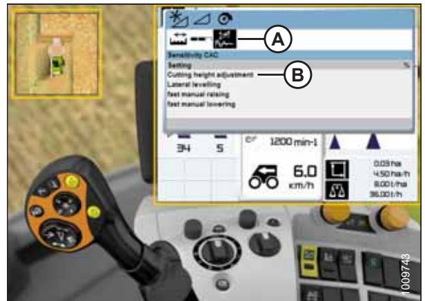
Figure 3.573: CLAAS Lexioni kombaini ekraan
