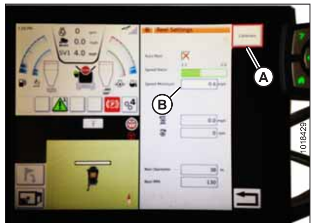
Figure 3.641: Trumli sätete kalibreerimine
