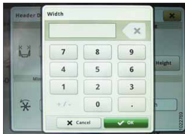
Figure 3.772: John Deere S700 ekraan – heedri laiuse seadmine
