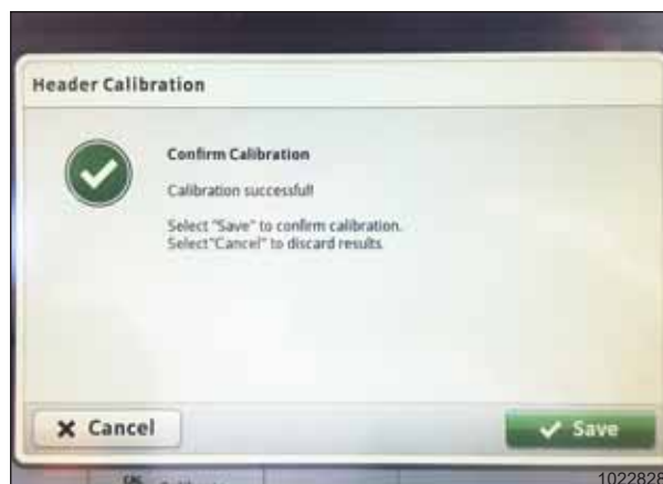
Figure 3.800: John Deere S700 ekraan – heedri kalibreerimine
