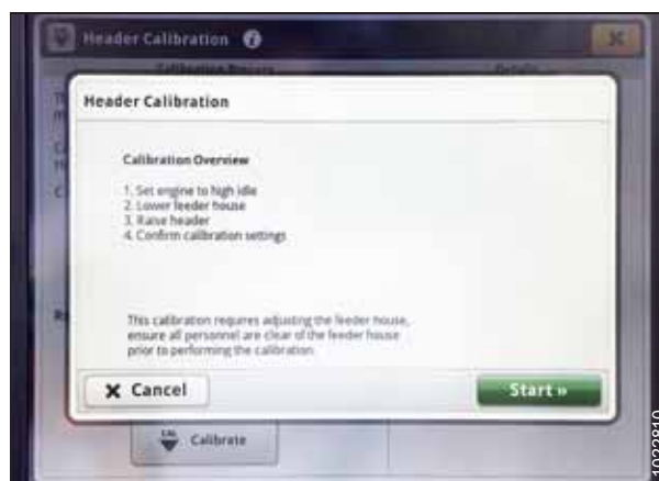
Figure 3.799: John Deere S700 ekraan – heedri kalibreerimine
