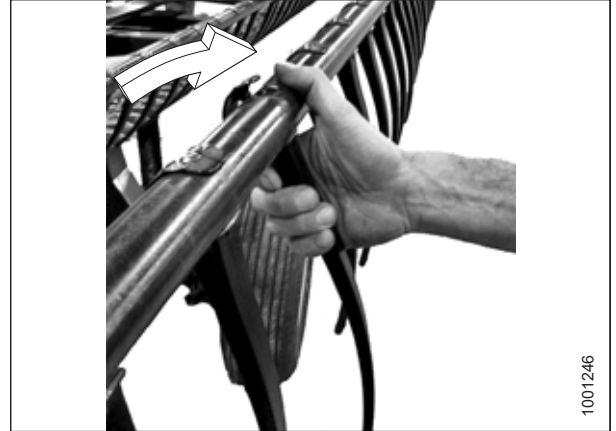
Figure 4.276: Installing Plastic Finger
