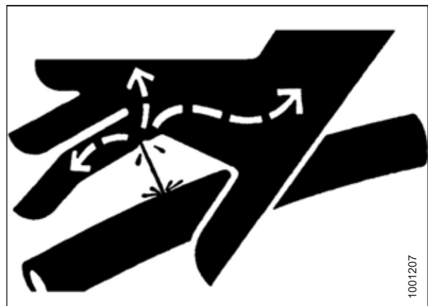
Figure 4.1: Hydraulic Pressure Hazard
