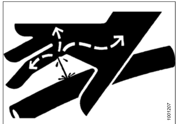
Figure 1.12: Hydraulic Pressure Hazard
