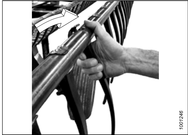
Figure 4.281: Installing Plastic Finger
