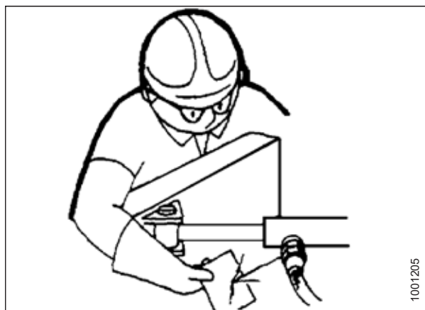
Figure 4.2: Test de fuites hydrauliques
