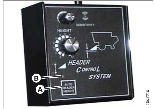
Figure 4.125: Combine Header Control System
