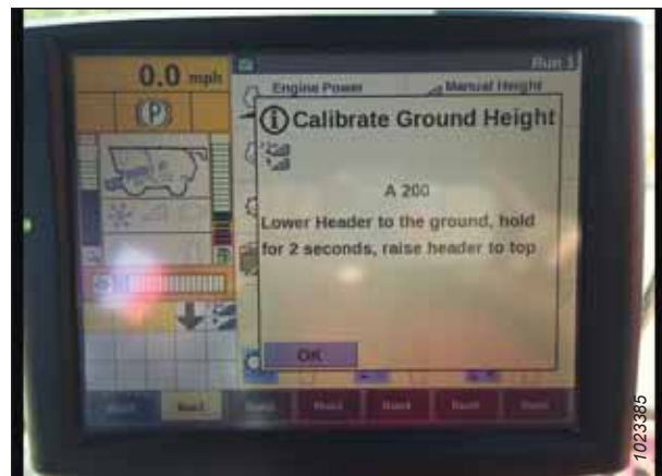
Figure 4.32: Calibrating Auto Header Height
