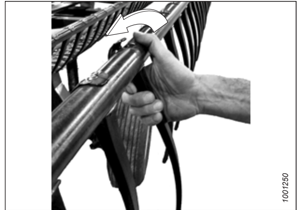
Figure 6.274: Removing Plastic Fingers
