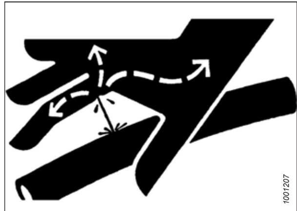
Figure 1.12: Hydraulic Pressure Hazard
