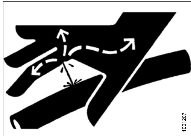
Figure 1.12: Hydraulic Pressure Hazard
