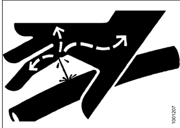
Figure 5.3: Hydraulic Pressure Hazard
