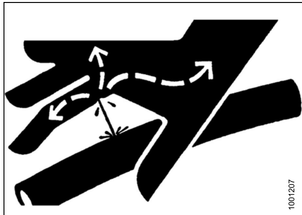
Figure 1.12: Hydraulic Pressure Hazard
