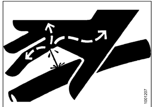
Figure 1.12: Hydraulic Pressure Hazard
