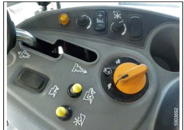
Figure 4.47: Height Adjustment Knob on the Combine Control Console
