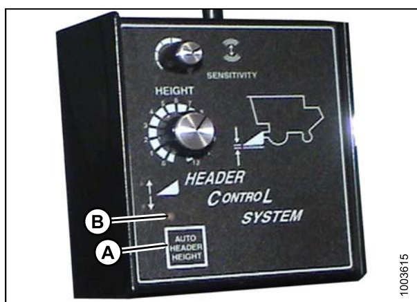
Figure 3.147: Combine Header Control System
