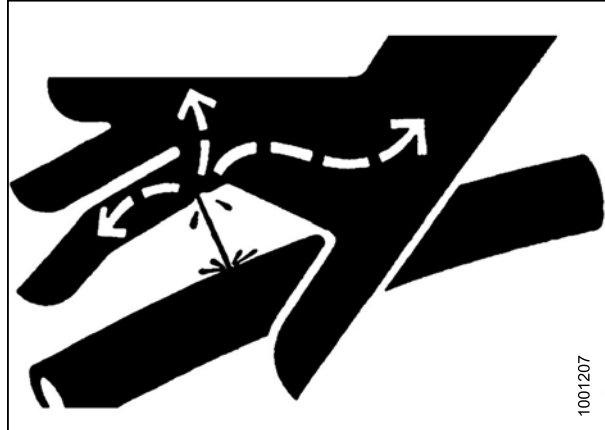
Figure 5.2: Hydraulic Pressure Hazard
