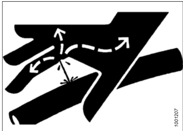
Figure 5.1: Hydraulic Pressure Hazard
