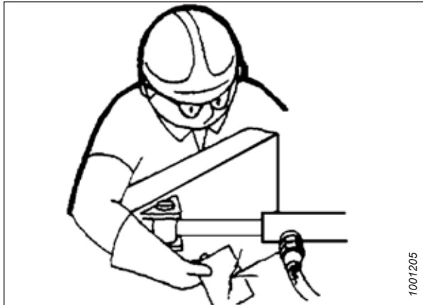
Figure 4.2: Test de fuites hydrauliques
